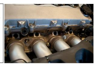
11. NOTE: If installing on a Supercharged Exige-S with intercooler, some grinding is required of the intake manifold's aluminum boss as circled in the picture.
