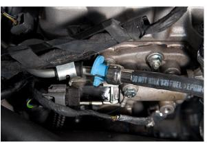
4. Carefully remove the fuel rail with the injectors still attached.
