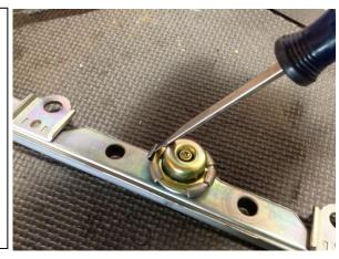
6. When all the tabs are bent out of the way, pull the pulse damper out by pulling straight out. Do not pull unevenly or pry from one side, as this may distort pulse damper.
