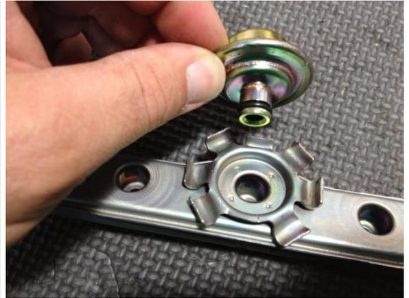
7. **To prevent failure, lightly lubricate the o-ring on the damper and install into the center port on the Radium fuel rail.**
