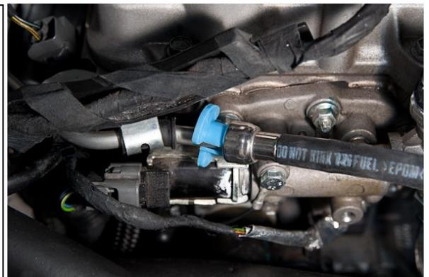
4. Carefully remove the fuel rail with the injectors still attached.
