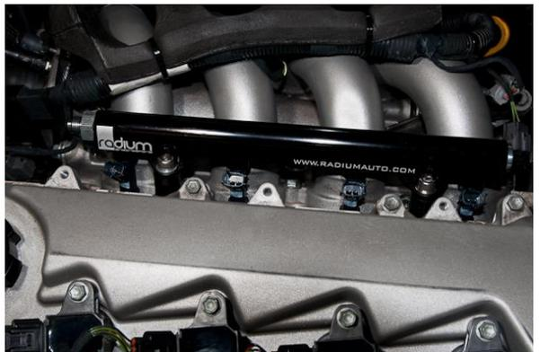
13. If installing 20-0012-00 or 20-0012-PK, the OEM fuel feed line will be reused. When tightening the hose to the fuel rail, hold the fuel rail fitting in place with a wrench. This avoids over-stressing the fuel rail mounting tabs.
