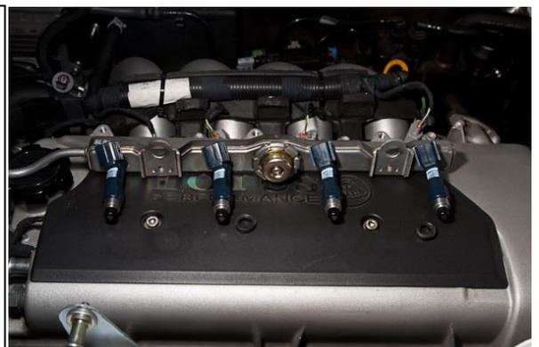
5. On the OEM fuel rail, locate the fuel pulse damper. Gently pry up on the tabs that hold it in place.
