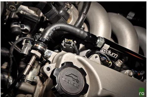
14. Connect the battery and turn the ignition switch to the ON position (without starting the engine) to allow the fuel pump to prime the system.
