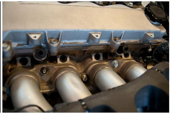
11. NOTE: If installing on a 2-Eleven or supercharged Exige-S with intercooler, some grinding is required of the intake manifold's aluminum boss as circled in the picture.
