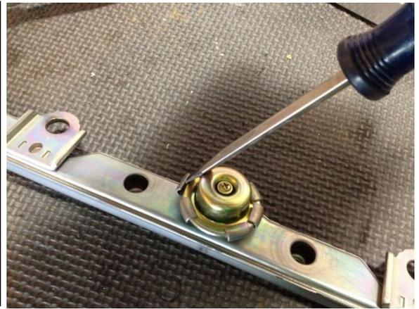
6. When all the tabs are bent out of the way, pull the pulse damper out by pulling straight out. Do not pull unevenly or pry from one side, as this may distort fuel pulse damper.
