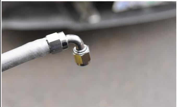
7. Torque the B-Nut on each hose end to the catch can fittings.
