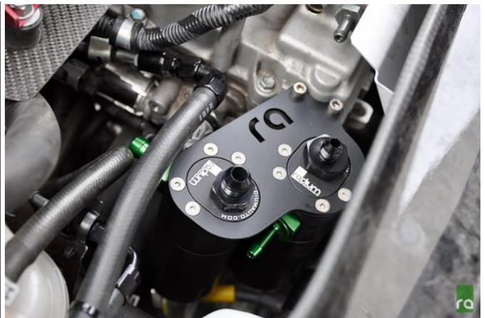
6. Using oil, lubricate the hose end barbs and force each hose onto the respective hose end (as shown). Next, screw the small 90 degree hose (shown) onto the appropriate catch can top fitting. Do not tighten yet. Slide a clamp on and push the hose onto the smaller (PCV valve) barb fitting on the valve cover. NOTE: It might be helpful to loosen the bolts that hold the catch can bracket to the valve cover. This will allow some movement of the catch cans to help get the hoses in place.
