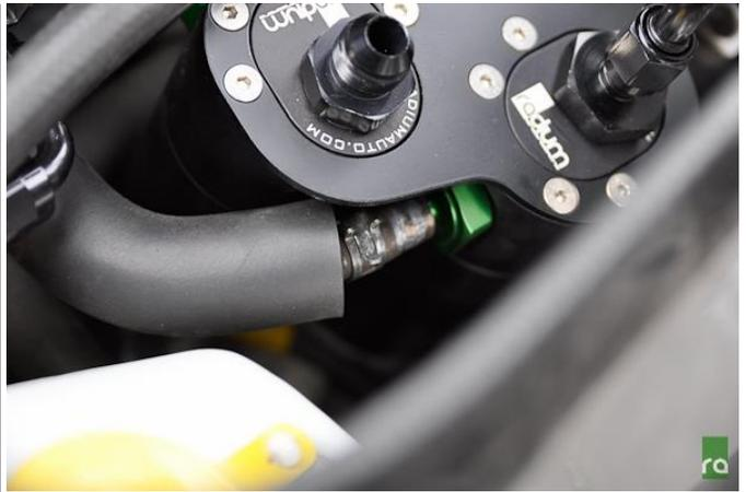
9. The larger PCV hose that was removed in the earlier steps is going to be cut down and used between the port on the throttle body and the larger barbed fitting on the forward most catch can.
