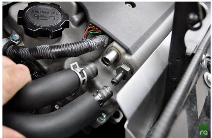
3. Disconnect the larger PCV hose the same way from the port on the throttle body (shown) and remove the hose from the engine bay.
