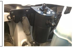
2. Either port can be used as the inlet or the outlet. Flow direction is not critical. The inside diameter of the hose used should match the factory hose. NOTE: Before installing the adapter fittings, lubricate the O-rings with engine oil.
