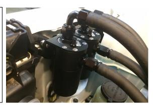
3. Using the oil dipstick, check the fluid level occasionally. If any oil registers, properly dispose by either unscrewing the bottom plug or unscrewing the bottom half of the catch can(s). If the vehicle is regularly tracked, the dipstick should be checked more frequently. A 10mm deep socket can be used to remove the dipstick if tight.
