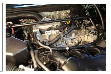
10. Using the included zip ties, secure the three hoses, that are routed along the top of the engine, to the fuel rail.
