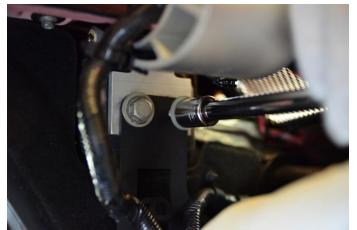
5. Using the 8 included M5 countersink screws, secure both catch cans to the mounting bracket. It is recommended to use Blue Loctite thread-locker on these fasteners.
