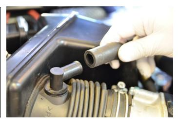
7. Locate the other end of the hose from the previous step where it attaches to the rear valve cover. Use pliers to release the hose clamp and remove the hose from the valve cover fitting. Pull the hose out from underneath the intake manifold, as shown to the right. Rotate the hose ~180 degree with respect to this port (pointing toward front of car) and reattach the hose and clamp to the fitting on the valve cover.
