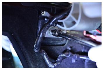
3. To install the Radium catch can mounting bracket, first insert the previously removed hinge bolt though the left mounting hole.
