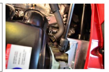
8. Locate the other PCV hose that connects the intake manifold port to the front bank PCV port, shown at right. To disconnect this hose follow the same procedure as the previous step.
