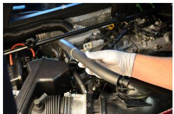
9. Cut a section of the included 3/8" ID hose to roughly 32" long. Route it from the LEFT catch can side port (use supplied hose clamp) to the intake manifold port (use factory hose clamp).
