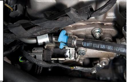
3. Release the retaining clip securing the pipe joint to the header tank bracket. Slide the orange colored safety lock to allow access to the connector release button. Push the release button and gently pull this hose assembly out and away from vehicle.
