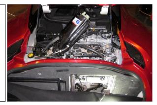
10. It is advised to plug (or tape over) all 6 cylinder intake ports to prevent objects from falling down into the engine.
