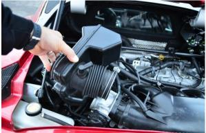
5. Locate the coolant hoses at the throttle body. Using a pair of pliers, squeeze the spring clamps (a) and slide them down the hose a few inches. Prepare the area for coolant to be spilled with shop towels. Carefully, pull these hoses off the throttle body barbs, and plug each hose quickly to avoid spillage.
