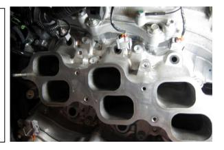
15. If installing 20-0198-PK or 20-0198-00, rotate and point the SAE quick disconnect fitting (as shown) towards the fuel tank. Push the OEM fuel tubing over the billet fitting until a positive click is felt.
