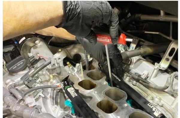
23. For Toyota 2GR-FE engines which use the additional engine braces, modify the brace (shown) with a cut-off wheel in the area illustrated.
