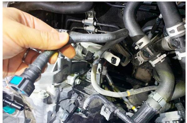
28. As shown, fully insert the OEM feed line to the SAE quick connect until a "click" is felt.
