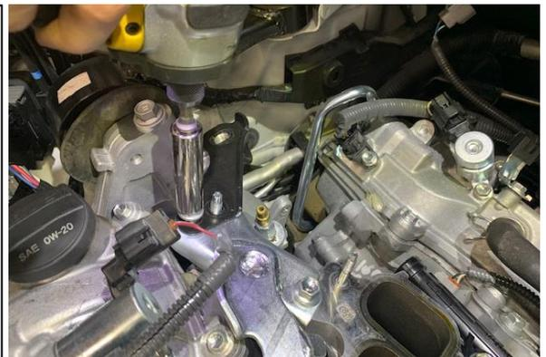
12. On the opposite side of the engine, pull the electrical stay up off the stud shown.
