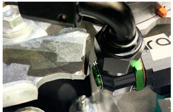
25. For those using the Radium Engineering plumbing kit, temporarily install the provided PushLok hose ends to the fuel rail end port fittings. Lineup the included hose and cut to length. Every application is different, but 5 inches (127mm) is typically best.
