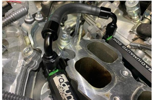
27. For those using the Radium Engineering plumbing kit, pop off the OEM fuel feed line from the plastic stay on the engine. This will free up the OEM line.
