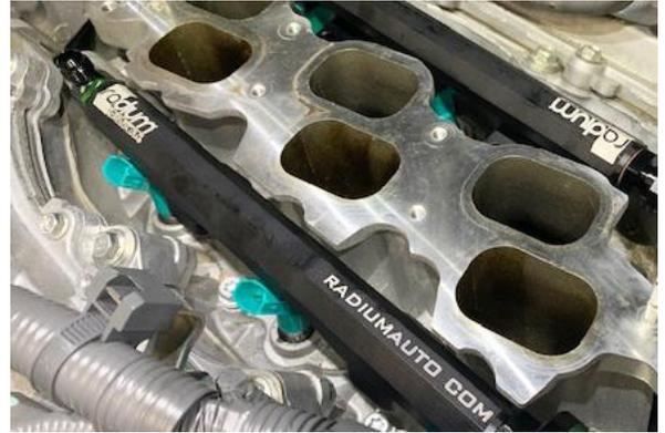
22. Fasten down the fuel rails using the included M8 bolts and washers and a 5mm Allen wrench.
