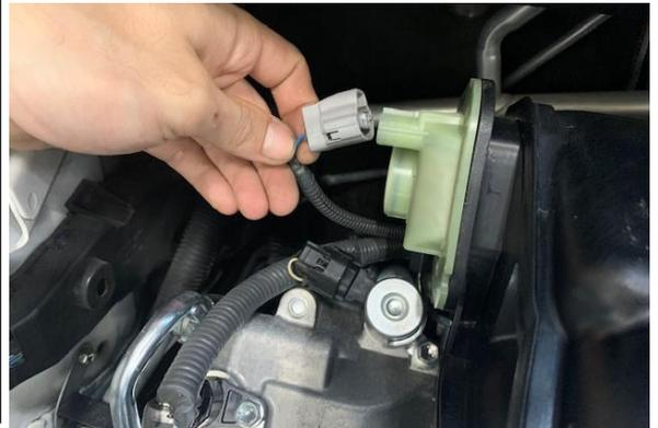
8. To access the fuel rails, the upper intake plenum must be removed from the lower intake manifold.
