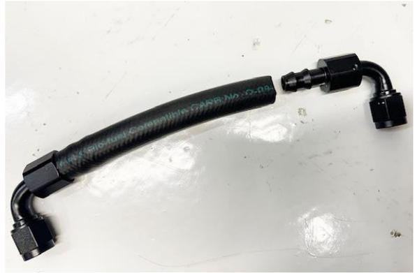
26. Using a non marring 9/16" aluminum wrench, tighten the 6AN hose ends.
