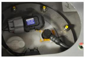
5. The Radium Engineering fitting was designed to be as low profile as possible for maximum clearance reasons. If not already assembled, torque the fitting to the hose end that will be used. **CHECK THE GAP BETWEEN THE HOSE END NUT AND FITTING HEX (as shown).** If there is not a gap, the hose end B-nut has potentially bottomed out on the Radium fitting before sealing on the flared surface.
