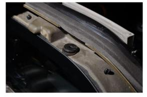
C. Remove the fuel filler bezel and hose from the fuel filler neck. The hose will be attached to the sub-frame. Cut the cable zip-tie to free up the hose. Remove the three Phillips head screws from the back side.
