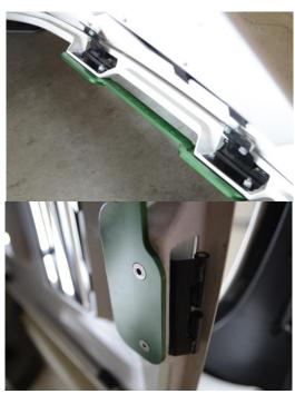
G. After all of the screws in the brace are tight, apply a piece of the included hook and loop (Velcro) to each pad on the brace, as shown.
