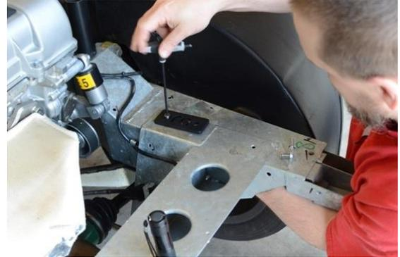
N. With clamshell still off the car, the foam roll bar cover on the interior can be installed. But first, two slots will need to be cut into the cover where the 2 Allen bolts screw into the bottom side of the upper portion of the clam shell.
