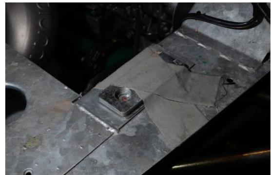
B. Locate the shim washers at the upper mounting holes, above the rear window near the roll bar. Remove these shims. These will not be reused.
