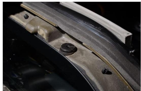
C. Remove the fuel filler bezel and hose from the fuel filler neck. The hose will be attached to the sub-frame. Cut the cable zip-tie to free up the hose. Remove the three Phillips head screws from the back side.
