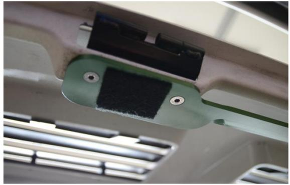
H. Apply the mating Velcro pieces to the two locations on the firewall that the deck lid hinges originally attached to, just below the rear window.
