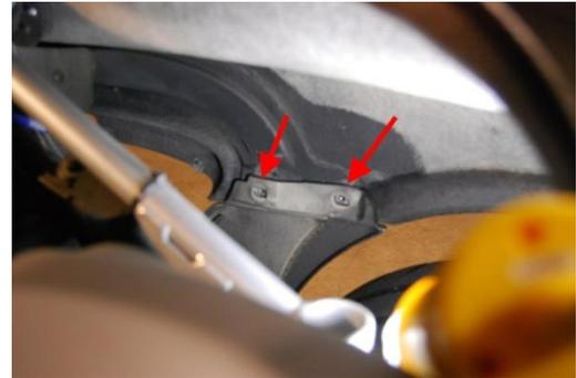
26. Position yourself near the rear wheel well. Have a helper stand at the opposite wheel well. Gently lift up on the wheel well lip and lift the clam up off of the car. Check to make sure there are no parts snagged or fasteners that are still installed.
