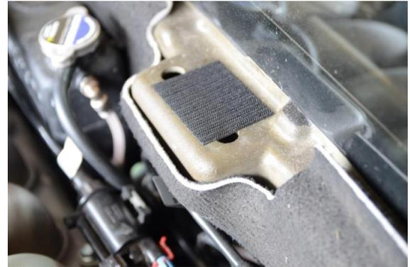
I. Locate the four black aluminum shim plates in the kit. Lay them out in the locations of the previous taped-on factory steel shims as shown. Note: your shims make look slightly different from the ones shown in these instructions.
