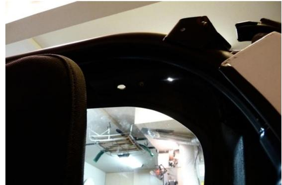
O. Luckily the cover's underside already has a molded edge (line) drawn for you to cut along. A hand held rotary tool such as Dremel is good to use for this step. Use a multi-purpose cutting bit.
