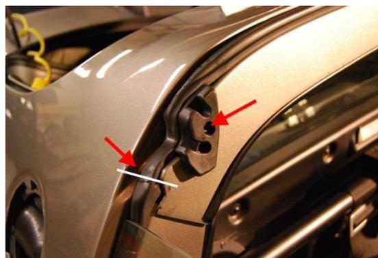
20. From inside the car, reach around behind the roll bar to the back side of the clamshell circled in the picture. Remove the 10mm head M6 bolt from this area. One per side. These will not be reinstalled.
