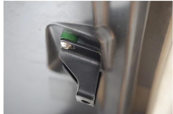
F. Locate the billet aluminum deck lid hinge brace and associated hardware. Install the deck lid with the brace as shown. Insert the included M6 countersunk screws from the bottom. Place the included M6 washers down first.
