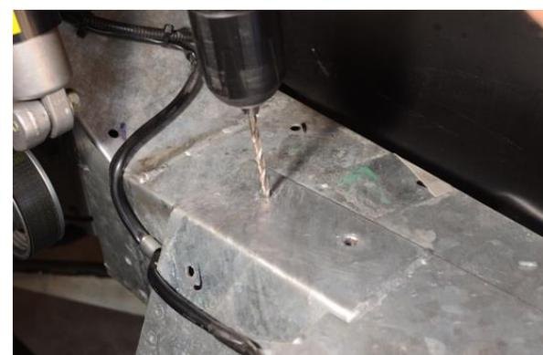
L. Insert one of the included flat-head Allen bolts through the shim and into the hole drilled in the previous step. Ensure that the large hole in the shim lines up with the threaded hole in the frame. If not, a larger may be in order. NOTE: The shims in some kits may look different than what is shown in these pictures, however functionality is the same.
