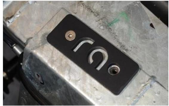
M. Reach your hand, or use a long wrench, into the frame rail and install one of the included lock nuts to the bolt inserted in the previous step. A trick is to use a closed end 10mm wrench and tape one of the sides to encapsulate the nut. Tighten the bolt. Do this at all four locations.
