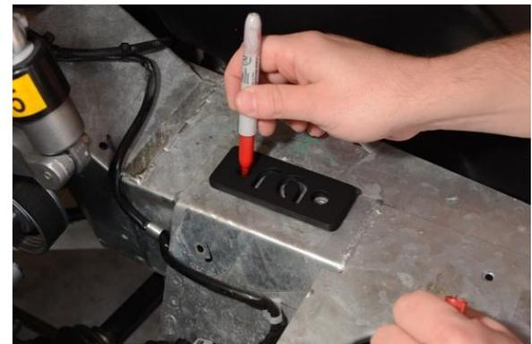
K. Drill holes at the locations marked with the pen. Start with a small drill bit and work your way up to a 9/32" drill bit.
