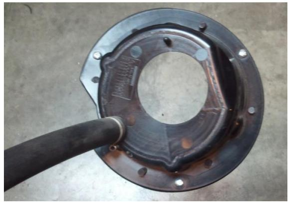
D. Separate the bezel into two pieces. On early models these are attached with an adhesive. Simply pry the 2 apart with a flat head screw driver or a chisel.
