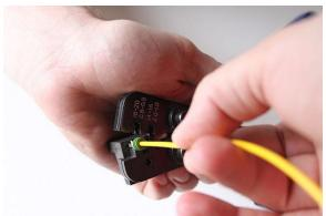
After the terminal has been crimped, the ratcheting mechanism of the crimping tool will release and allow the tool to open, releasing the crimped terminal/wire.
