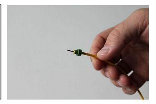
Slip the already stripped wire and seal assembly into the terminal. The smaller portion of the seal should be inside the tangs of the terminal. That way once crimped, the tangs grab the seal and hold it tightly.
