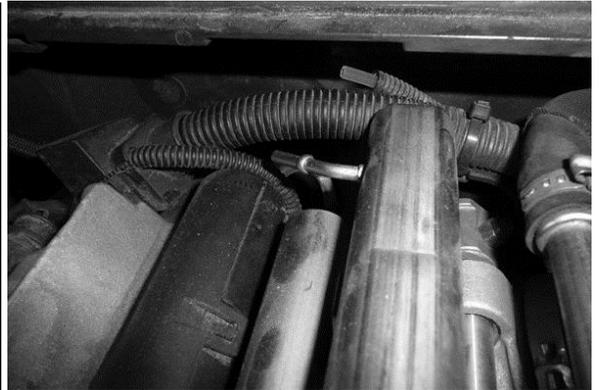
7. Because the new big bore fuel rail takes up more space, the barbed nipple will need to be slightly modified.
