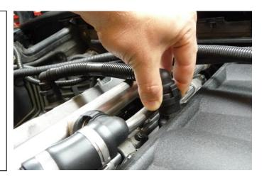
5a. The 05-06 M3 models have a secondary PCV system (shown). All of the modifications in these instructions apply for the 05-06 M3 models. However, when the valve cover fitting is spun around in the following steps, the small 05-06 convoluted tubing will stay intact and simply reroute accordingly.
