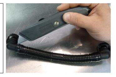
7. Cut a 19" section from included hose. Install between the valve cover and catch can top port. If installing the catch can back to the OEM intake manifold port, cut a 25" section from the hose. Install between the intake manifold and the catch can side port.
