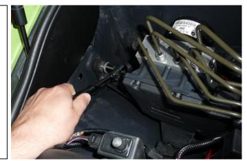
2. Install the mounting bracket to the 2 factory locations. For all models, use a 4mm Allen wrench and secure the included M6x1mm button head bolt to the boss near the ground lug, as shown.
