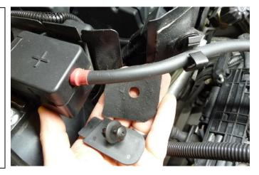
11. Slide the supplied clamps onto each hose and install the factory BMW plastic barb fittings. Lubrication may be required. To secure, use pliers and slide the clamps over each fitting. Press and lock both OEM fittings back into place.
