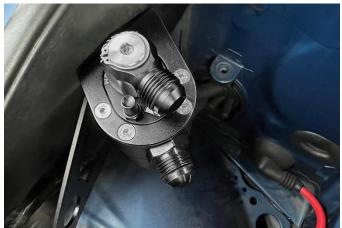
5. The factory 01-04 E46 M3 PCV tubing routes from the valve cover back to the intake manifold (pre throttle). The catch can hoses will be plumbed between these two connections. NOTE: See Step 5a below for the 05-06 M3's secondary PCV system.
