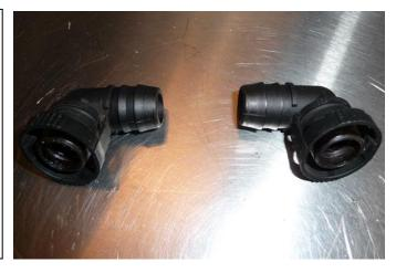
8. Each rubber hose will need 1 of the included hose ends installed. To assemble, simply lubricate the barbs of the included push-lok hose end. A drop of engine oil will suffice.
