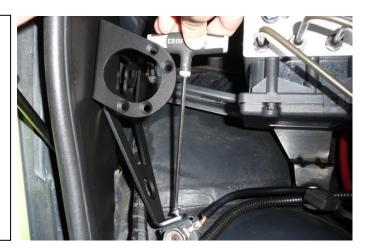
3. Lubricate the O-ring and tighten the straight adapter fitting into the side (outlet) port using an adjustable wrench. Install banjo fitting to the catch can top port.
