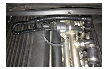
6. Next, it is necessary to remove the plastic convoluted tubing from the 2 barbed fittings.
