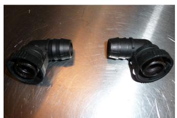
8. Each rubber hose will need one of the included hose ends installed. To assemble, simply lubricate the barbs of the included push-lok hose end. A drop of engine oil will suffice.
