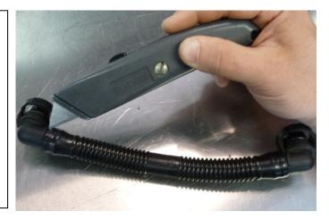
7. M3: cut a 19" section from included hose. Install between valve cover and catch can top port. If installing catch can back to intake manifold port, cut a 25" section from hose. Install between intake manifold and catch can side port.
