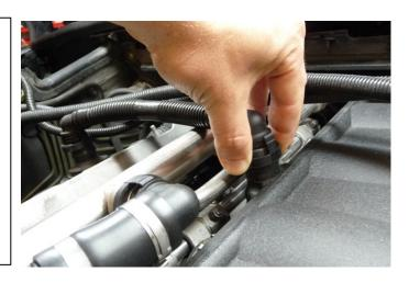
5a. The 2005-2006 M3 models have a secondary PCV system (shown). All of the modifications in these instructions apply for the 2005-2006 M3 models. However, when the valve cover fitting is spun around in the following steps, the small 2005-2006 convoluted tubing will stay intact and simply reroute accordingly.
