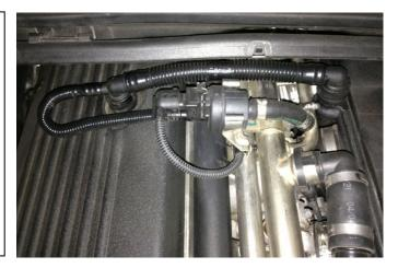
6. Next, it is necessary to remove the plastic convoluted tubing from the 2 barbed fittings. The BMW E46 M3 model is shown. Non BMW E46 M3 models will be slightly longer.
