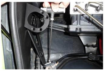
3. Lubricate the O-ring and screw the straight adapter fitting into the side (outlet) port.
