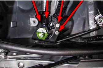
5. The factory 2001-2004 E46 M3 PCV hose routes from the valve cover back to the intake manifold pre throttle. The catch can hoses will be plumbed between these two connections. See Step 5a. below for the 2005-2006 M3's secondary PCV system.
