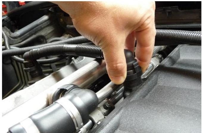
5a. The 2005-2006 M3 models have a secondary PCV system (shown). All of the modifications in these instructions apply for the 2005-2006 M3 models. However, when the valve cover fitting is spun around in the following steps, the small 2005-2006 convoluted tubing will stay intact and simply reroute accordingly.
