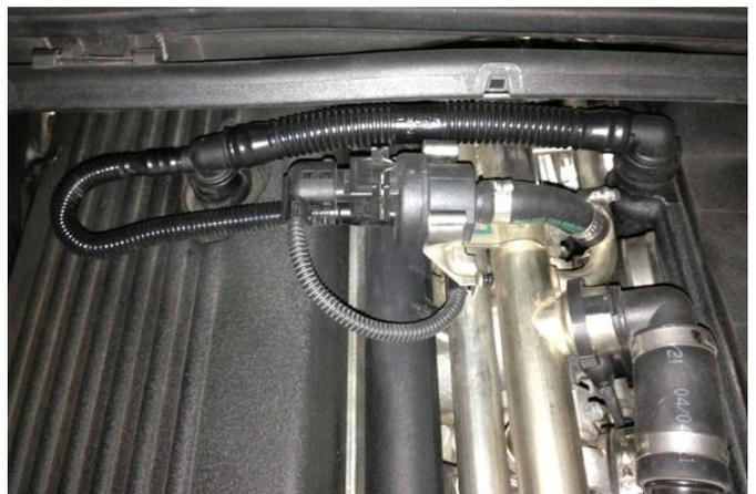
6. Next, it is necessary to remove the plastic convoluted tubing from the 2 barbed fittings. The BMW E46 M3 model is shown.
