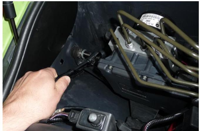
2. Install the mounting bracket to the 2 factory locations. For all models, use a 4mm Allen wrench and secure the included M6 button head bolt to the boss near the ground lug, as shown.
