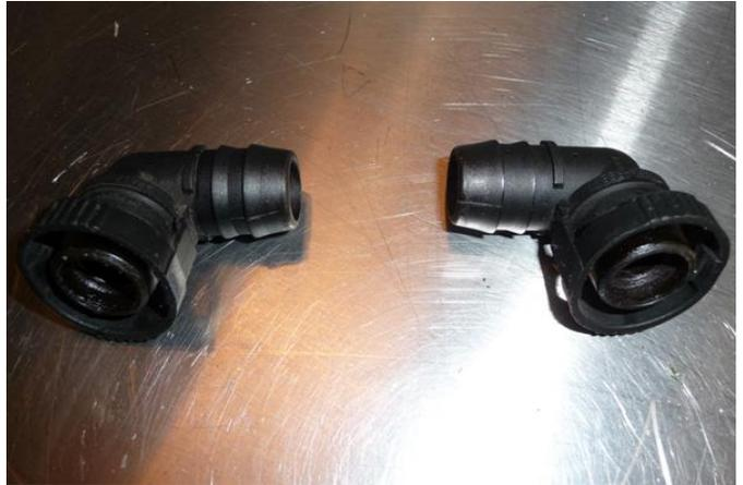
8. Each rubber hose will need one of the included hose ends installed. To assemble, simply lubricate the barbs of the included push-loc hose end. A drop of engine oil will suffice.
