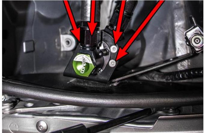
5. The factory 2001-2004 E46 M3 PCV hose routes from the valve cover back to the intake manifold pre throttle. The catch can hoses will be plumbed between these two connections. See Step 5a. below for the 2005-2006 M3's secondary PCV system.
