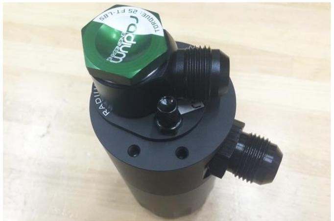
4. Check that the catch can's bottom port is plugged or close the optional petcock valve, if applicable.
