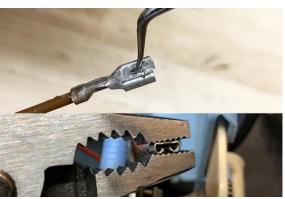
14. The picture at right shows how the spade terminals will properly lock together in later steps. Do not perform this step yet.
