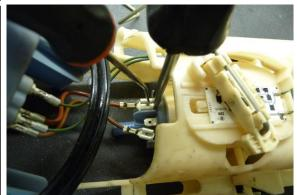
9. Pry the rubber isolation grommets off each side of the fuel pump using your fingers and a screwdriver, as shown. These will reinstalled later.
