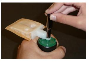
20. Position the new pump assembly back into the BMW hanger. Reinstall the rubber isolation grommets from the previous steps.
