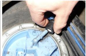
6. To remove the lock ring, there are many aftermarket tools that can be purchased. If not available, a rubber mallet and punch will suffice. NOTE: For the E36, the lock ring is plastic so be careful.
