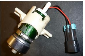
19. Locate the new fuel pump sock filter and the metal lock washer. Insert the sock onto the bottom of the pump. This installs only one way. NOTE: filter sock may differ than picture.
