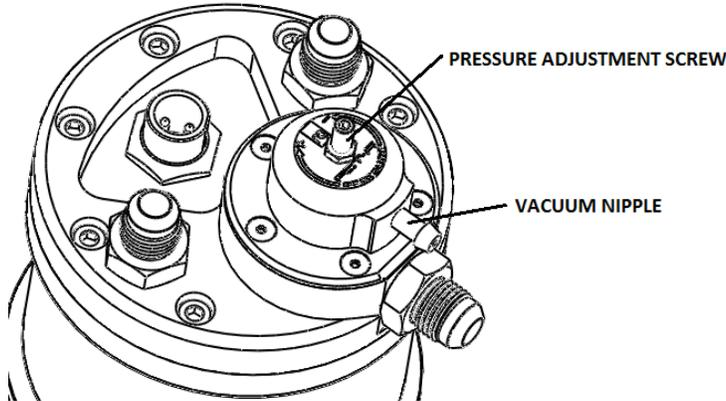
Re-install the FST pump fuse. Turn the ignition key ON. The lift pump and FST pump should prime at the same time. Check for leaks. Watch the pressure gauge during this time. Make adjustments to the pressure adjustment screw using a 3/32" Allen wrench, until proper fuel pressure is obtained. Several priming cycles may be necessary to allow an adjustment and reach the desired pressure.
