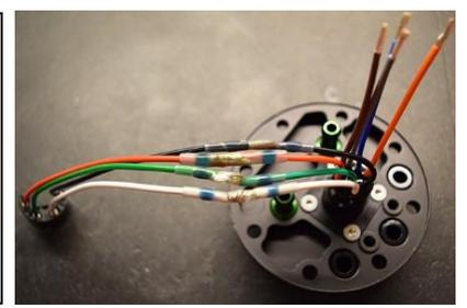
3. As shown, the Ti Automotive E5LM has 4 electrical terminals.
