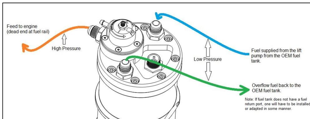
The FST-R has three -6AN ORB ports, these ports come by default with 6AN male adapters installed. Other adapters can be used as well but must be purchased separately. To complete the installation, -6AN (3/8”) hoses will need to be constructed. The two -6AN ports on top of the fuel surge tank (shown in blue and green) are interchangeable. One port receives fuel from the main tank’s “lift” pump and the other port is for fuel returning back to the main fuel tank. The side port on the FST-R
