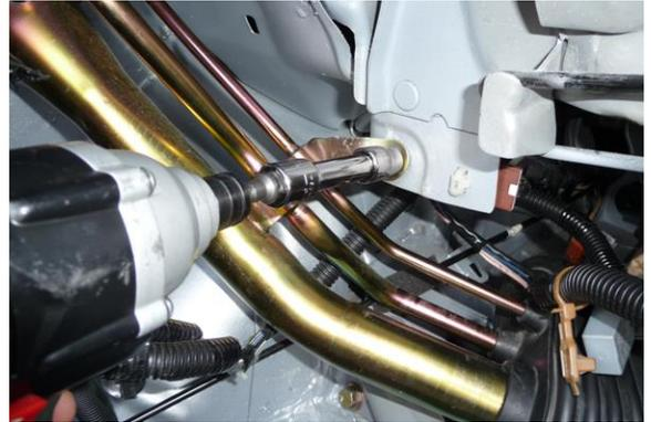
7. From the trunk area, pull the gas filler inwards to release the 3 studs from the body.
