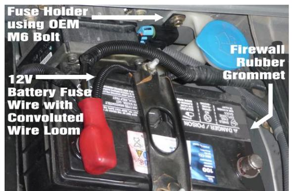
33. Use the convoluted wire loom for the trunk wiring, as shown. Reconnect the battery.
