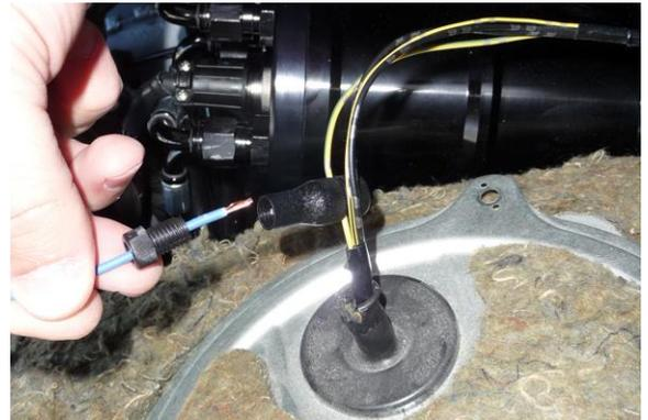
30. Insert the blue wire through the center section of the Posi-Tap connector. Screw the Posi-Tap connector together and give the wire a quick tug to make sure it seated properly.
