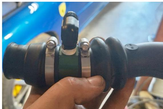
23. 06-09 kit: Route the other short Radium hose from the port fitting closest to the top of the FST (upper left) to the fuel filler -6AN male fitting installed in the previous step. (06-09 kit not shown)
