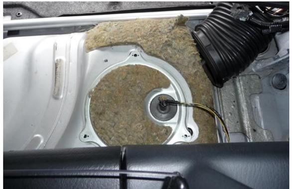
14. The center port on the 2000-2005 S2000 fuel pump hanger is the drain back from the FPR back to the OEM tank. The other port (shown lower right) connects the OEM pump to the fuel rail. Note: The 2006-2009 S2000 only has this fitting.
