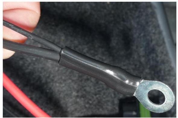
29. The FST pump's relay trigger will be tapped from the OEM fuel pump's yellow/green strip power wire.
