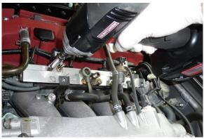
8. Carefully pull the fuel rail out of the vehicle. Have a rag handy as there will be excess fuel still remaining in the fuel rail.
