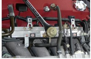
6. Use a 10mm socket wrench to remove both M6 bolts which hold the 2 hard vacuum line brackets.
