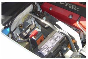
3. Using a pair of pliers, release the OEM spring clamp from the PCV valve hose found on the valve cover. Carefully pull the hose off the PCV valve barb.
