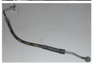
18. Find the female inverted flare to -6AN male adapter fitting in the kit. Screw and secure it to the Radium PTFE hose.
