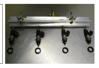
10. For 2004-2005 models, use a T30 Torx wrench to remove and discard both M6 bolts that secure the banjo bolt flange to the OEM fuel rail. To release, pull the banjo bolt flange away from the fuel rail.
