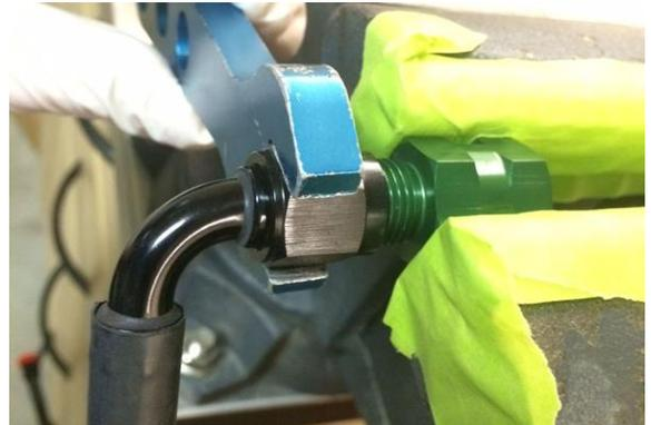
18. From underneath the vehicle, mate the inverted flare fittings. Route the PTFE hose upwards staying clear of hot and/or moving parts. Secure to the -6AN male fitting on the top port of the fuel rail.
