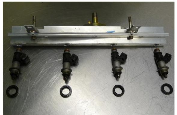
10. Install the OEM FPR to the Radium fuel rail using the OEM hex head bolts. Inspect the O-ring for damage or tears. Replace if necessary. The FPR screen from the OEM rail will not be reused.
