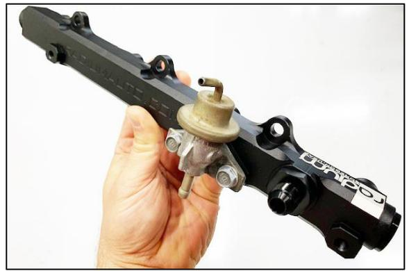
11. Find the supplied 5/32" vacuum hose. Cut in 2 sections to replace the discarded hard tubes. If rerouting is unclear, use the schematic shown for help.
