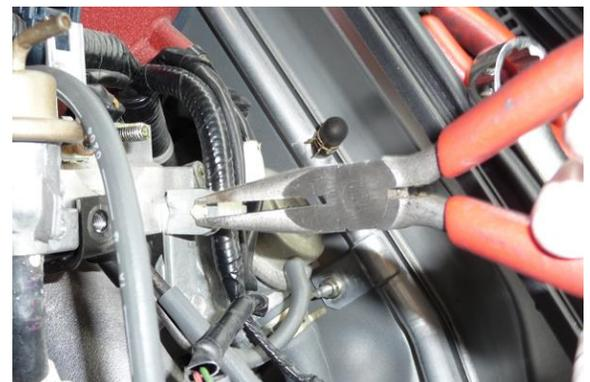
5. Use a 22mm wrench to loosen the pulse damper banjo bolt shown. Some fuel may spill out of this connection so have a rag handy. Pull the banjo off the threaded stud.
