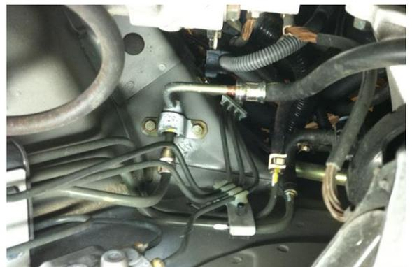
15. Using a 10mm socket wrench and extension, remove the two M6 bolts that secure the fuel feed line clamp to the chassis, as shown. These will not be reused.
