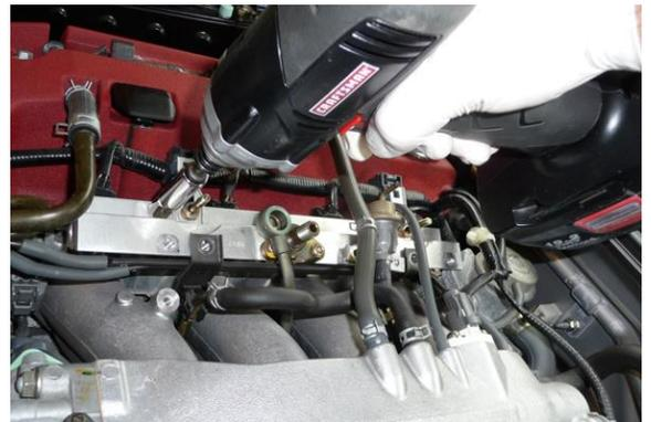
8. Unclip the fuel injector wiring harness from the 2 stays. Unplug the fuel injector connectors and carefully pull the fuel rail out of the vehicle. Have a rag handy as there will be excess fuel still remaining in the fuel rail.
