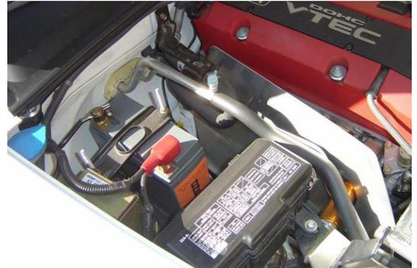
3. Using a pair of pliers, release the OEM spring clamps from the PCV valve and crankcase breather hoses found on the valve cover. Carefully pull the hose off the PCV valve barb.
