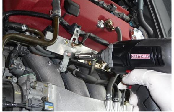
7. Using a 10mm socket wrench, remove the four M6 bolts that secure the two mounting brackets that attach the fuel rail to the intake manifold runners. These two brackets will be reused.
