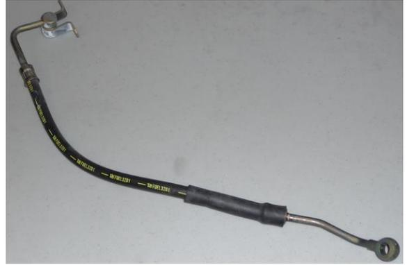
17. Find the female inverted flare to -6AN male adapter fitting in the kit. Screw and secure it to the Radium PTFE hose.
