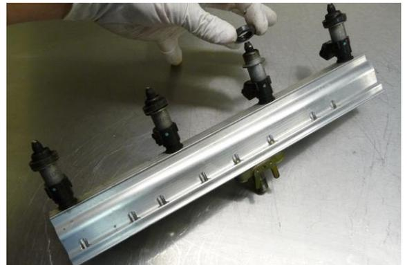
9. Gently pull each fuel injector from the OEM fuel rail. Inspect all O-rings and grommets for rips and tears and replace, if necessary. **Lubricate the O-rings when reinstalling injectors into Radium fuel rail.**
