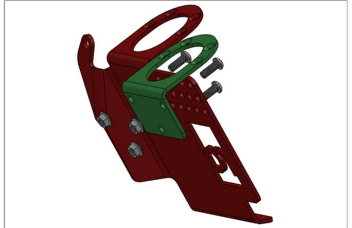
9. Set the coolant overflow reservoir bracket back in its normal location, but do not reinstall the 2 bolts.
