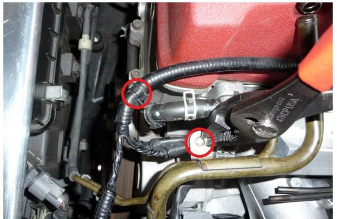
2. Using the pliers, squeeze and release the spring clamp on the hose that attaches to the valve cover breather nipple.
