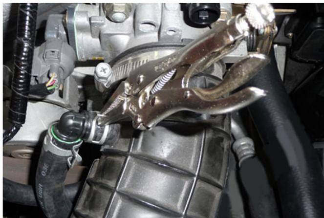
17. Route the catch can's top port hose under the throttle body staying clear of moving parts. Albeit a tight fit, the 1/2" hose and OEM spring clamp can squeeze onto the valve cover barb, as pictured. Tighten the hose ends to the catch can using a 7/8" wrench (preferably a non marring wrench).
