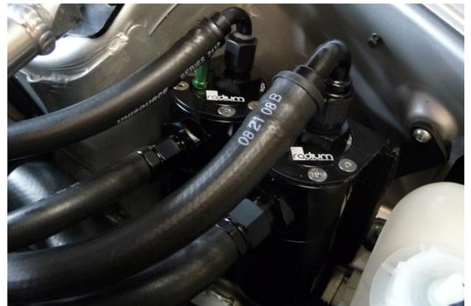
22. Using the oil dipstick, check the fluid level occasionally. If the vehicle is regularly tracked, the dipstick should be checked frequently. Properly dispose the oil by either unscrewing the bottom half of the can(s) or using the optional petcock valve if purchased.
