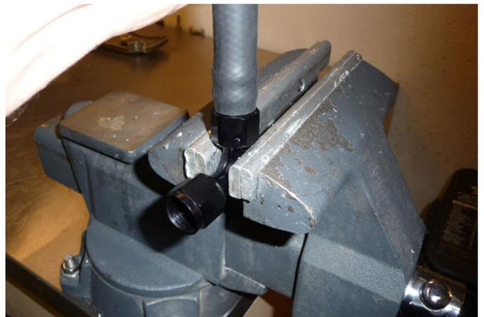
15. For OEM air intake systems, insert the included 90 degree barb to barb connector into the opposite end of the side port hose.
