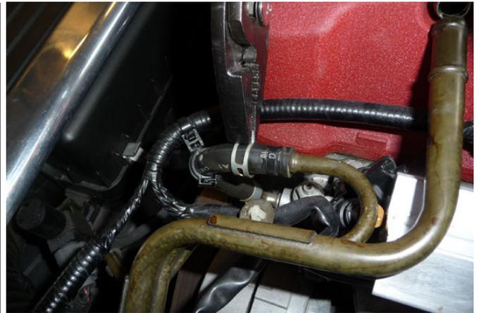
4. On S2000 models that have the early Honda Secondary Air Control Valve system, carefully pull the front two lower air control valve system vacuum lines downward and off the metal tube assembly, as shown.
