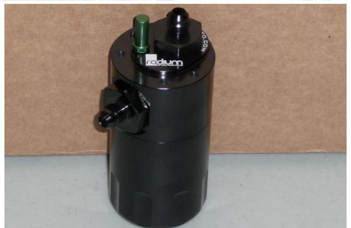
11. If the PCV catch can was purchased, find the 2 included -6AN male to -10AN port fittings. Install each into the PCV catch can's ports, as shown.
