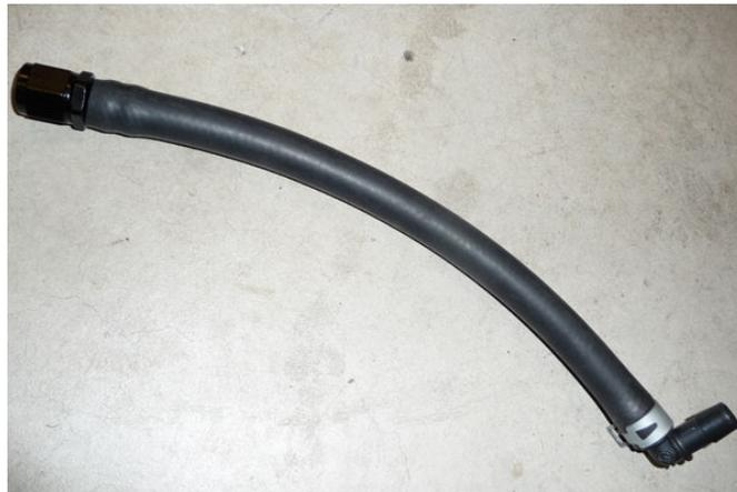
16. When routing the top port hose, make sure it will not come in contact with the serpentine belt on the front of the engine.
