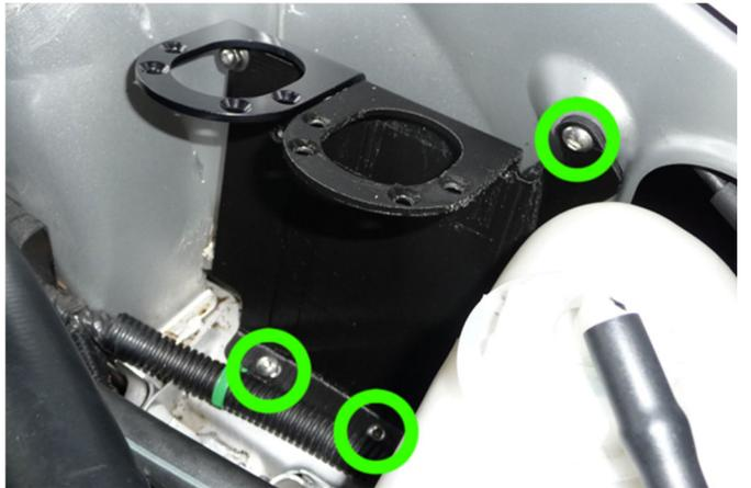
10. Using the 2 included -8AN male to -10AN port fittings, install into the crankcase vent catch can's ports, as shown.
