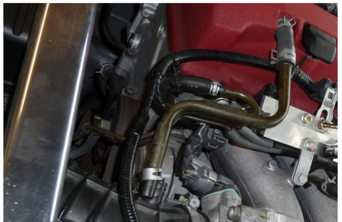
3. Use a pair of pliers to squeeze and slide both the spring clamps down the 5/16" coolant hoses that connect to the metal tube assembly barbs.
