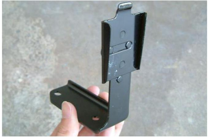
8. If the PCV and Crankcase Vent catch cans were both purchased, attach the 2 included catch can brackets together using the 3 sets of button head bolts and flange nuts.
