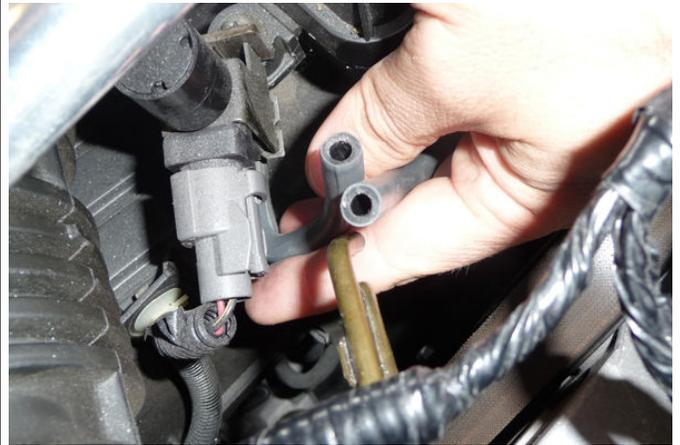
5. Remove the metal tube assembly from the vehicle (early model shown). This will not be re-used.
