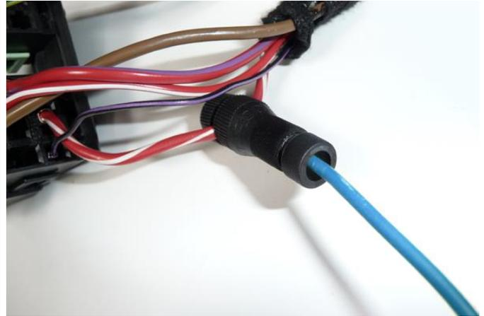
6. To properly use crimpless solder butt connectors, strip the wire insulation back and insert a wire through one side and then twist the 2 wires together. Next, center the connector on the bare wires and use a heat gun to melt the solder. Be careful with the surrounding area as the internal solder can take awhile to melt. Finally, verify the connection is solid by gently tugging.
