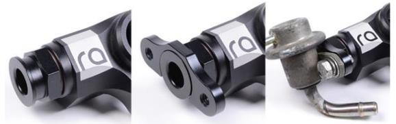
14. If using the 20-0112-10 or 20-0112-PK install the -6AN adapter into the inlet port of the fuel rail, as shown. ***If installing as part of the Evo X Fuel Delivery System, construct the fuel rail as shown in "Configuration 4" at the bottom of this document.***
