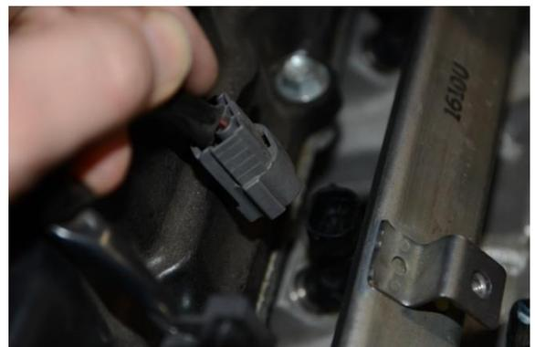
9. Use a 12mm socket and remove the two M8 bolts securing the fuel rail to the intake manifold. These bolts will not be reused.
