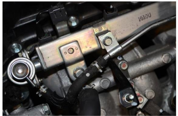
5. Remove the two M6 screws holding the fuel return hard line to the fuel rail. This bolts will not be reused.
