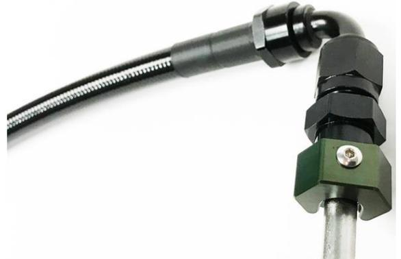
20. Install the 45 degree hose end to the fuel rail inlet port using the supplied -6AN male fitting and an 11/16" wrench.
