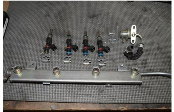
13a. If the fuel rail was produced before December 2016, the end port (shown) of the fuel rail is threaded for 3/8" NPT (tapered pipe thread). The adapter fitting must use PTFE (Teflon) paste on the threads. Hand tighten, then add another 1.5 to 3 turns with a wrench.
