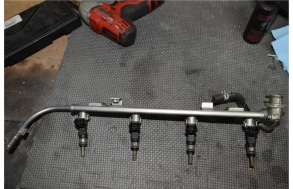
11. Be careful to not lose or drop the plastic mounting boss spacers in the engine bay. These will be required for the Radium Engineering fuel rail.
