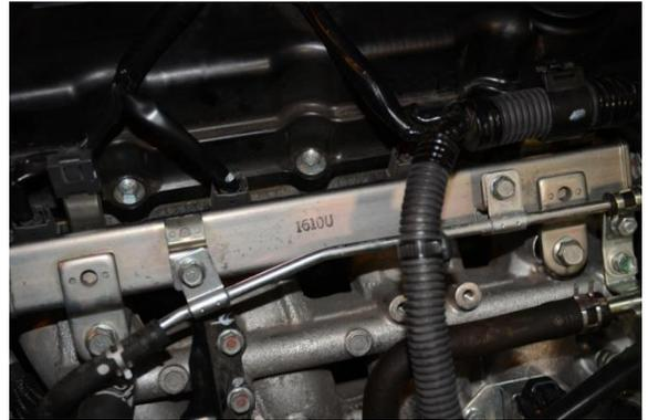
6. Remove the M6 nut and screw for the third bracket holding the fuel return hard line. Remove the small bracket. This will not be reused. Replace the M6 screw and tighten.
