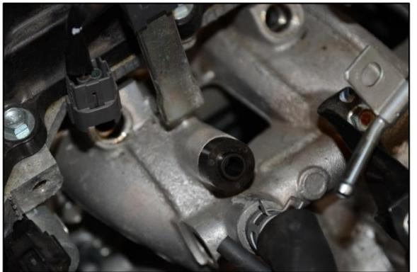
12. Remove the fuel injectors and fuel pressure regulator from the stock fuel rail. NOTE: The fuel injector clips cannot be reused on fuel rails produced prior to September 2017.
