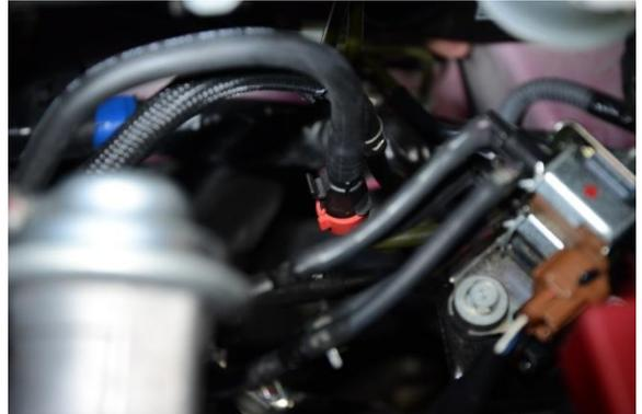
2. Locate the other end of the fuel hose at the fuel rail hard tube. Another red clip is used here. Use a small tool to pull the red clip to the open position, as shown. Disconnect the fuel hose from the fuel rail hard line. Remove the fuel hose from vehicle.
