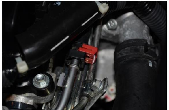
3. On the intake manifold, remove the two M6 bolts holding the black sheet metal bracket. Unclip the wiring harness from the bracket and remove the bracket.
