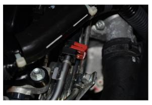
3. On the intake manifold, remove the two M6 bolts holding the black sheet metal bracket. Unclip the wiring harness from the bracket and remove the bracket.
