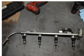
11. Be careful to not lose or drop the plastic mounting boss spacers in the engine bay. These will be required for the Radium Engineering fuel rail.
