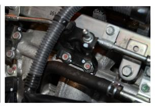
4. Pull the vacuum hose off the fuel pressure regulator barb (left side of picture).
