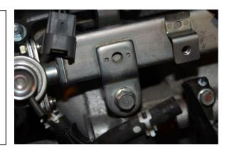
10. Remove the fuel rail from the vehicle. It will contain fuel. Drain excess fuel into a safe container for disposal.
