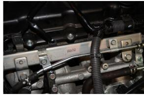
6. Remove the M6 nut and screw for the third bracket holding the fuel return hard line. Remove the small bracket. This will not be reused. Replace the M6 screw and tighten.
