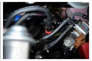
2. Locate the other end of the fuel hose at the fuel rail hard tube. Another red clip is used here. Use a small tool to pull the red clip to the open position, as shown. Disconnect the fuel hose from the fuel rail hard line. Remove the fuel hose from vehicle.
