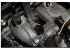
12. Remove the fuel injectors and fuel pressure regulator from the stock fuel rail. NOTE: The fuel injector clips cannot be reused on fuel rails produced prior to September 2017.
