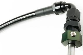
20. Install the 45 degree hose end to the fuel rail inlet port using the supplied - 6AN male fitting and an 11/16" wrench.
