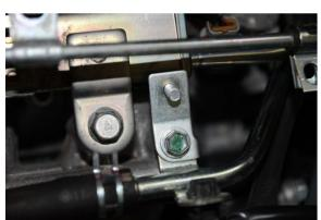
7. Remove the cushion clamp from the fuel return hard line that remains from the previous step. The rubber sleeve is left in place on the hard line.
