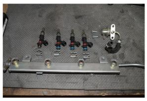
13a. If the fuel rail was produced before December 2016, the end port (shown) of the fuel rail is threaded for 3/8" NPT (tapered pipe thread). The adapter fitting must use PTFE (Teflon) paste on the threads. Hand tighten, than add another 1.5 to 3 turns with a wrench.
