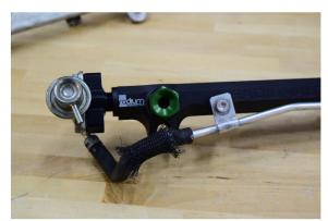
16. Lubricate each fuel injector's top O-rings with engine oil. Fully insert the fuel injectors into the Radium fuel rail injector ports.
