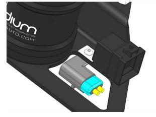
7. Place the fuel surge tank assembly into the location shown and line up the mounting holes.
