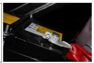
25. For the chassis ground connection, use the location where the negative battery cable attaches to the trunk floor.
