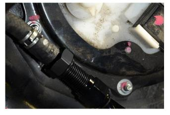
17. Locate the ¼" non-permeating rubber hose, 2 hose clamps, and the other -6AN to barb adapter in the kit.
