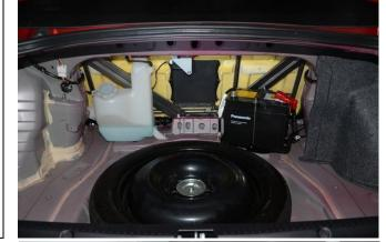
2. Remove the washer fluid reservoir lower mounting bolt shown in the picture. Note: This bolt will be replaced with one of the M8 Allen head bolts in the kit.
