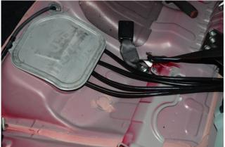
20. Make four marks on the cover where a passage for each hose will need to be cut.
