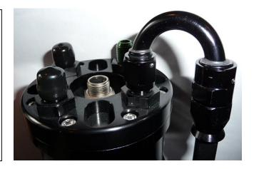
15. Locate the hose that is 41.5" long and has a 90 degree and a straight hose end fitting. Install the male quick-connect adapter into the straight hose end.
