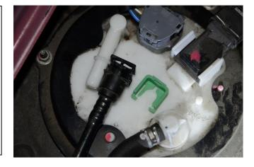
13. Locate the hose in the kit that does not have a hose end fitting on one end.
