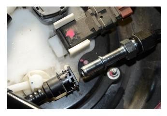
16. Install the included -6AN to hose barb adapter into the OEM fuel return hose, as shown. Re-use the spring clamp.
