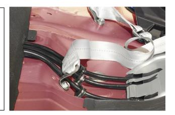
21b. EVOX FST install kits purchased after May 2016 come with a 5-Way Separator Clamp (Radium 20-0231), replacing the previously mentioned cushion clamps.
