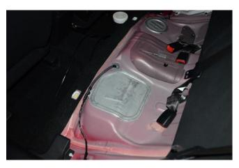
12. With the top of the fuel pump hanger exposed, clean the area with some water and a rag as it will be covered in dirt.
