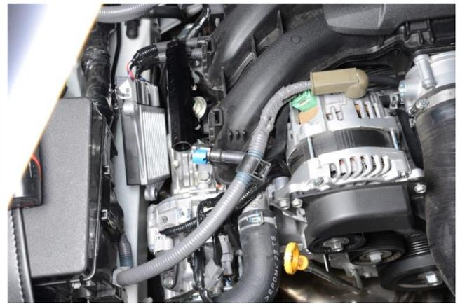
25. The black metal cover needs to be reused to provide mounting for the ECU. Modify it by cutting a large slot to clear the end fitting of the Radium fuel rail. This may take several test fitting iterations. CAUTION: Do not cut metal or create sparks near open fuel lines and gasoline.
