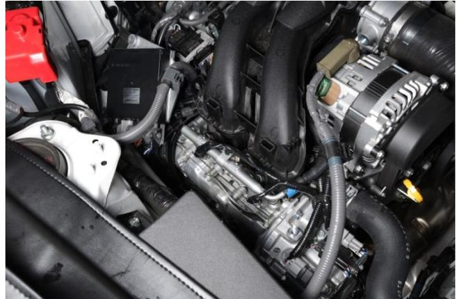
22. Unplug the electrical connectors for the two fuel injectors. Unlock the fuel cross-over hose by pulling out on the blue clip. Disconnect this hose from the fuel rail pipe.
