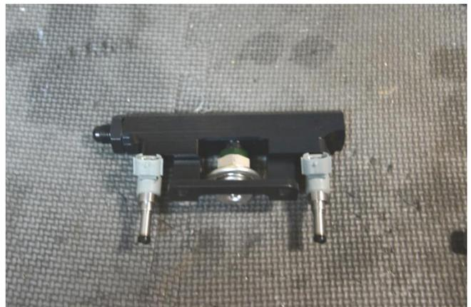
24. Install the fuel rail in place and reuse the factory M8 bolts in the mounting bracket.
