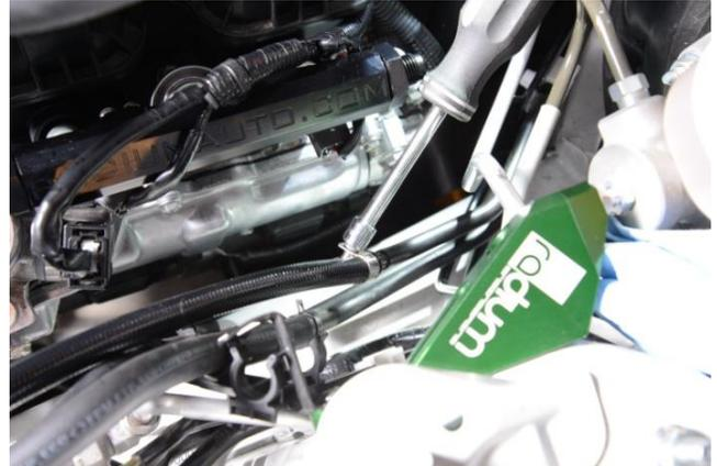
18. Connect the other end of the hose to the LH fuel rail front port. Secure the B-nut using a non-marring wrench. When tightening the B-nut, hold the fuel rail with a large adjustable wrench (or similar) to keep from bending the fuel rail mounting bracket. Use a rag or similar padding to keep the adjustable wrench from scratching the fuel rail.
