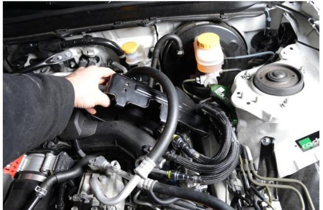
4. Locate the crossover fuel hose connection on the front of the LH fuel rail. The hose end fitting has a blue clip.
