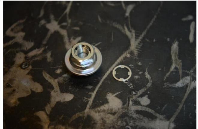
10. For 20-0111-PK or 20-0111-00 is used, install the fuel pulse damper adapter into the center port of the Radium fuel rail. **To prevent failure, the O-ring MUST be lubricated prior to assembly.**
