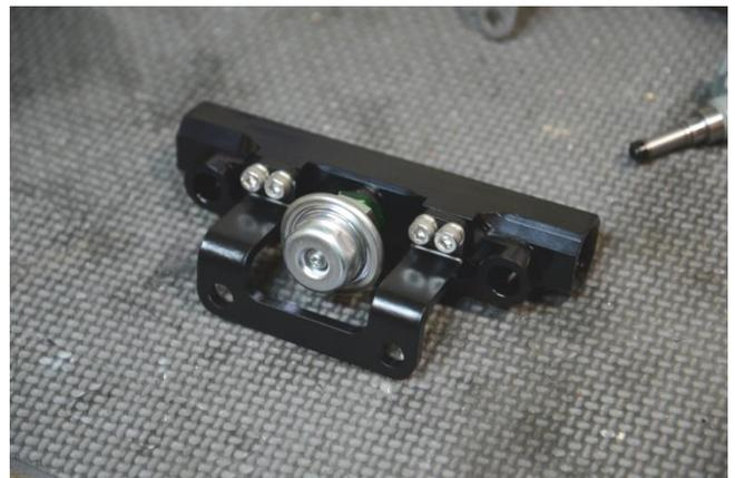
12. For 20-0111-00 or 20-0111-PK, install the included -6AN adapters into each end of the fuel rail, as shown. **To prevent failure, all O-rings MUST be lubricated prior to assembly.** Hold the fuel rail in a vice with non-marring jaws, and tighten the fittings with a 1" non-marring wrench.
