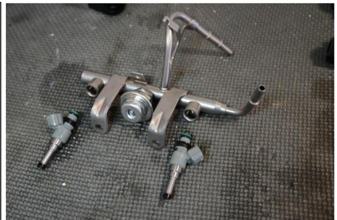
8. Secure the fuel rail in a vice and remove the fuel pulse damper using a 7/8" or 22mm wrench.
