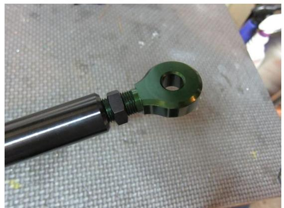
5. Place the bar into the engine bay and line up the rod ends to the large mount/gusset assembly holes vertically. **IMPORTANT: when inserting the rod ends into the brackets make sure the machined (bright silver) surface of the green anodized rod end is facing DOWNWARDS.**
