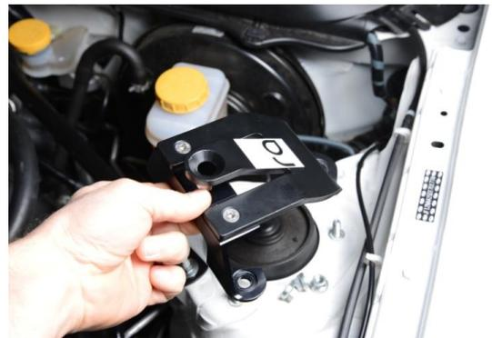
3. Place each mount/gusset assembly over the studs on top of each front strut tower.
