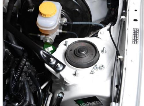
2. Using a 4mm Allen wrench, assemble each billet mount to a gusset bracket using the small stainless steel countersink screws.
