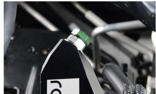
3. Fasten the master cylinder brace to the strut tower using the M6 screws included with the kit.
