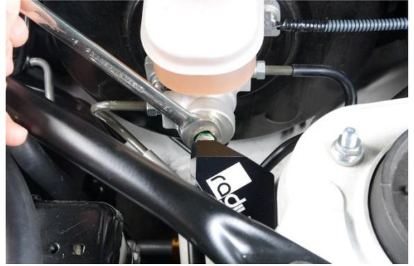
5. Using a 1/2" wrench, tighten the jam nut, as shown. Make sure the bolt does not turn when tightening the jam nut.
