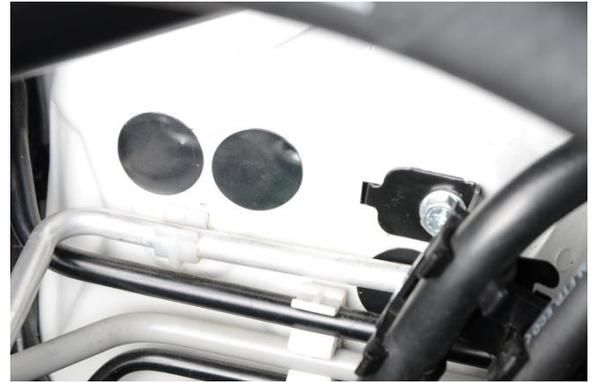
1b. For automatic transmission vehicles, the steel wire loom mounting bracket (shown) must be permanently removed. Use a 10mm socket wrench to remove the OEM M6 bolt.
