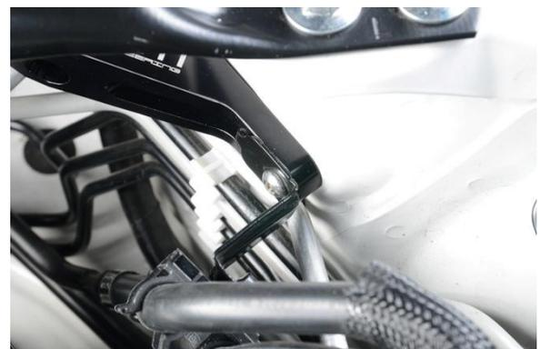
4. Using a 1/2" wrench, unscrew the bolt installed in step 2.
