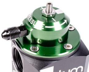
The vacuum nipple on the MPR can be unscrewed and replaced with a -3AN male adapter as shown in this picture. This adapter is available from Radium Engineering, part number 14-0369.
