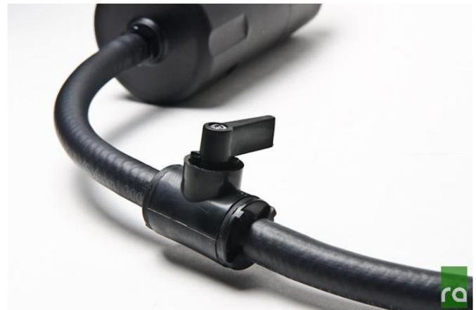
7. Use the oil dipstick to check the fluid level occasionally. If the vehicle is regularly tracked, the dipstick should be checked frequently. Properly dispose the oil by either unscrewing the bottom half of the can(s) or using the optional petcock valve (if purchased).
