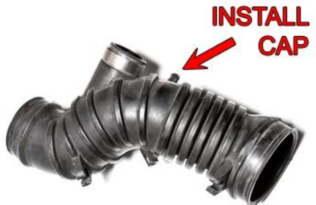
31. For applications that are still using a MAF sensor, the PCV hose should be removed. If not removed, a very small amount of "unmetered" air will enter the system through the catch can's breather filter. Install 1 of the included vacuum caps to the PCV valve (shown) and another vacuum cap to the intake manifold barb (not shown).
