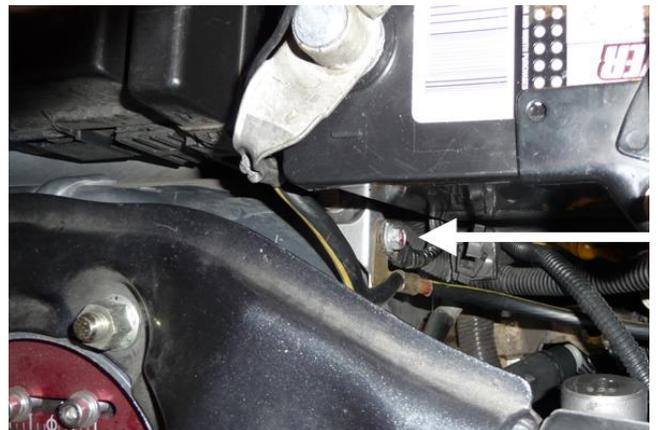
11. Route the large 10AWG red wire along the left side of vehicle connecting 1 fuse lead to the relay in the trunk. This wire is hot so stay clear of chaffing areas and secure appropriately. Use the crimp-less solder butt connectors and a ring terminal to secure to the battery 12V+ terminal.
