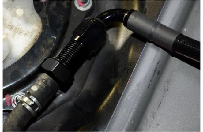
21. Locate the non-permeating ¼" ID rubber Barricade hose and the other -6AN male to barb adapter fitting in the kit.
