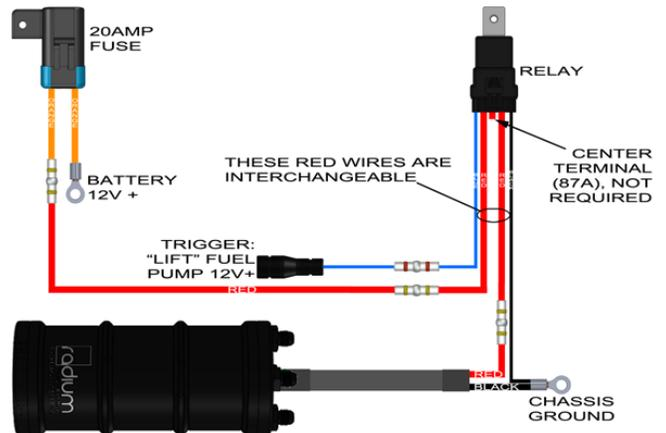
7. Permanently mount the relay and temporarily mount the grounding ring terminal of the large brace using the hardware included in the kit, as shown. Note: Both components mount on the front side of the brace (closest to the rear seat).
