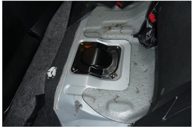
5. Release the fuel pump connector by squeezing the lock with your thumb and simultaneously pulling upwards.
