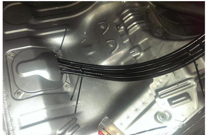
26. The hose routing will look similar to what is shown. Notice how the hoses go around the backside of the V-brace.
