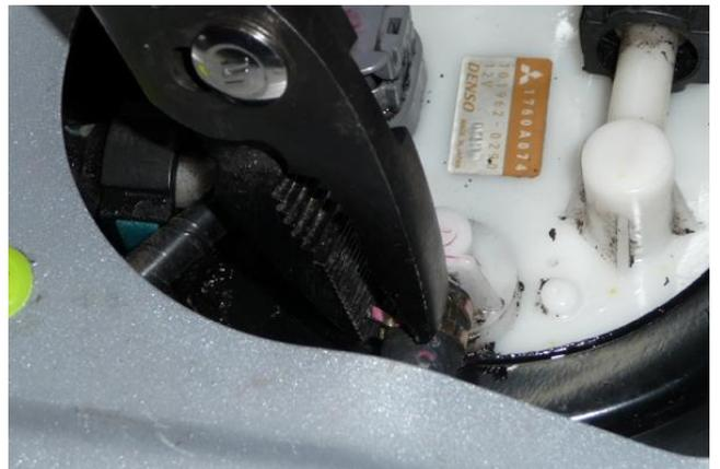
18. Locate the hose in the kit that doesn't have a hose end on one end. Using the included hose clamp, install the female quick disconnect fitting found in the kit, as shown.
