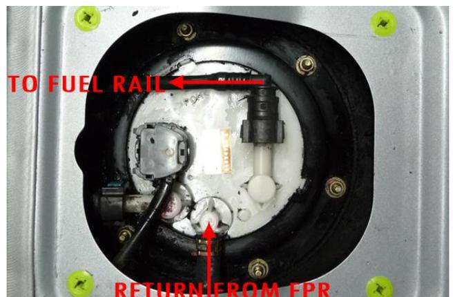
16. Remove the high pressure line from the fuel pump hanger fitting by first squeezing the 2 opposing tabs and then pulling away from the fuel pump hanger fitting.
