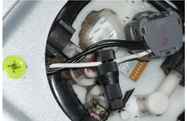
10. Find the fuse holder in the kit and confirm there is a 20A fuse installed. Using a 1/4" drill bit, enlarge the plastic fuse holder mounting bracket's hole.
