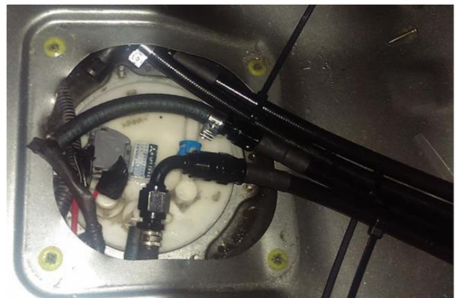
24. With the four hoses routed, test fit the OEM fuel pump access cover. Make a mark on the cover to cut away a section for the hoses and trigger wire to pass through, as shown.
