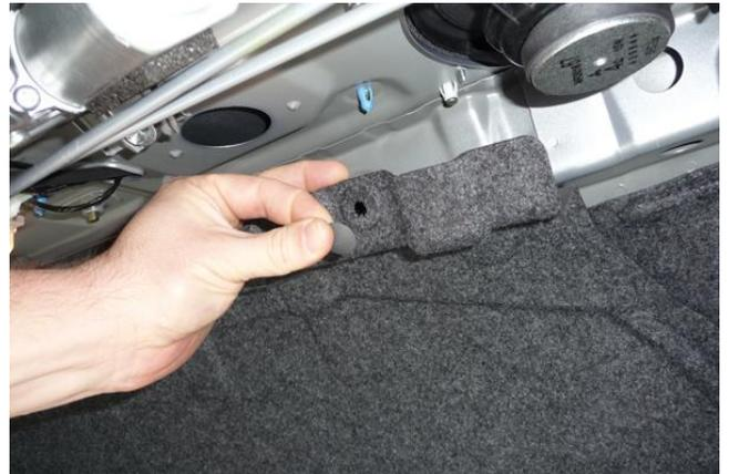
2. Remove the panel attached to the back of the rear seat from the vehicle, as shown.
