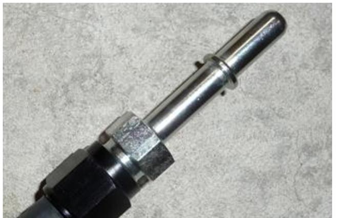
20. Locate the 40" long PTFE hose with 90 degree hose ends on both sides. Secure one of the included adapter fittings (hose barb to -6AN male) to one of the ends of the PTFE hose.
