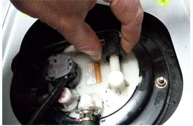
17. Loosen the spring clamp on the return hose with a pair of pliers, as shown.
