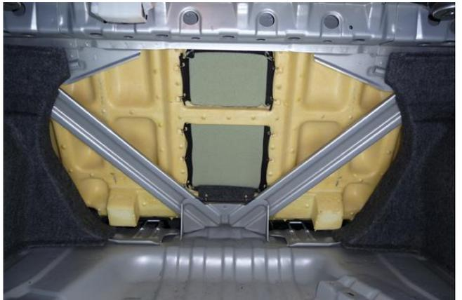
3. Lineup the large flat brace included in the kit to the support beams. Confirm the brace is horizontal using a level.
