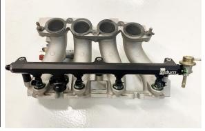
9. As a test, push the fuel injectors downward until they bottom out. Now inspect the injectors' upper O-rings and confirm they are still inserted into the fuel rail injector bores. Do not pressurize the fuel system until the proper height is achieved.
