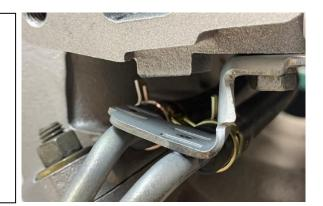
16. Measure the distance from the charge pipe barb to the Radium IACV spacer barb and cut the provided hose to length.
