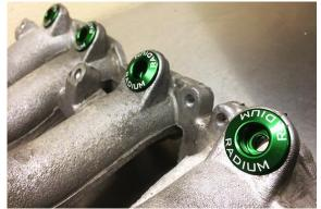
5. Install all fittings into the 3 ports (front, bottom, rear) of the rail. These are ¾-16 (8AN ORB). To prevent failure, lubricate all adapter port fitting O-rings.
