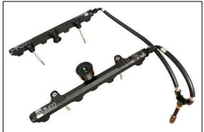
10. Here is the correct plumbing kit hose routing for the 2015+ (S550) Mustang.
