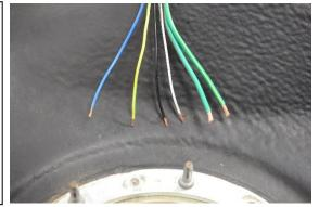
22. Insert a small piece of shrink tube onto each wire, then crimp on the ring terminals included in the kit. Use the 4 smaller ring terminals on the fuel level (and fuel temperature sensor wires if equipped). If powering a single pump using the OEM wiring (check power requirements), crimp the two larger terminals on the pump power and ground wires. NOTE: See the following step for additional details on powering a single pump.
