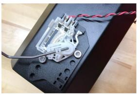
15. **Excluding Subaru FA20F vehicle applications:** Slide the OEM fuel level sender downwards onto the front of the collector box. Use the included bolt to secure the sender in place, as shown. Plug in the fuel level sender connector.
