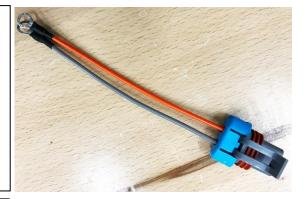
11. To install the fuel temperature sensor (if equipped), cut the 2 black wires at the white OEM connector allowing as much slack as possible. Strip the wires and crimp the 2 included ring terminals using a standard crimp tool.
