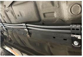
Push the -6AN (3/8") return fuel hose up into the engine bay. Position the end of the hose where the fuel pressure regulator return port is located. NOTE: This hose will be cut to length and terminated in later steps.
