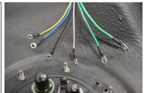
23. Connect the fuel temperature and fuel Level wires to the corresponding terminals on the pump hanger. The sensor wires do not have polarity, so they can be connected to either terminal.
