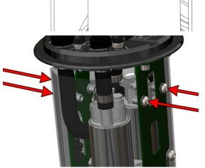
13. To connect the fuel level sender, cut the 2 wires at the OEM white internal connector allowing as much slack as possible. NOTE: One wire will be black and the other will be either yellow or red.
