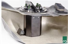
20. Install the OEM metal hold-down bracket and tighten all nuts to factory spec in an alternating cross-pattern.
