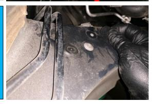
Using 14mm and 10mm wrenches, secure the fuel filter bracket to the chassis, as shown.
