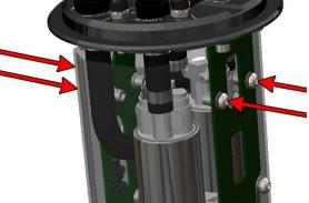
13. To connect the fuel level sender, cut the 2 wires at the OEM white internal connector allowing as much slack as possible. NOTE: One wire will be black and the other will be either yellow or red.
