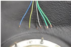
22. Insert a small piece of shrink tube onto each wire, then crimp on the ring terminals included in the kit. Use the 4 smaller ring terminals on the fuel level (and fuel temperature sensor wires if equipped). If powering a single pump using the OEM wiring (check power requirements), crimp the two larger terminals on the pump power and ground wires. NOTE: See the following step for additional details on powering a single pump.
