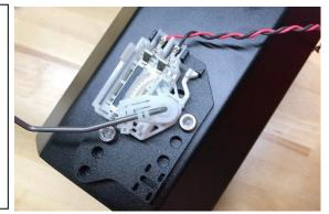
15. *Excluding Subaru FA20F vehicle applications:* Slide the OEM fuel level sender downwards onto the front of the collector box. Use the included bolt to secure the sender in place, as shown. Plug in the fuel level sender connector.
