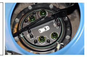
21. Cut off the OEM external 6-position fuel pump connector leaving as much slack as possible.
