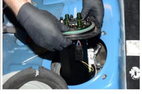
19. The top plate and gasket should be flush with the mounting ring.
