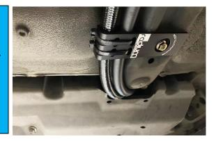
Near the fuel filter, secure the fuel lines using the provided cable zip ties. For LHD vehicles, pay close attention to the steering arm.
