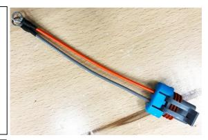
11. To install the fuel temperature sensor (if equipped), cut the 2 black wires at the white OEM connector allowing as much slack as possible. Strip the wires and crimp the 2 included ring terminals using a standard crimp tool.
