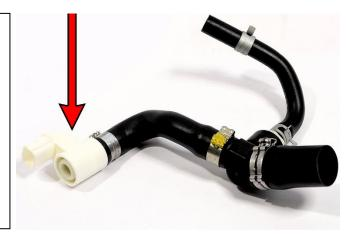
For aftermarket turbo inlets that do NOT support the OEM diagnostic connector, extra parts may need to be purchased. All that matters is that this port on the turbo inlet must be blocked off or plugged in some manner.
