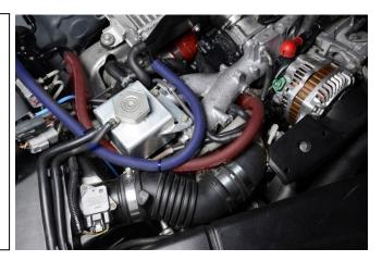
Cut a  $\frac{1}{2}$ " section out of the hose shown. This cut should be made just behind the coolant tank. Next, install the provided TEE fitting in line with the branch of the TEE pointing toward the throttle body.
