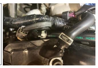
Install the provided plastic 90 degree elbow into the top portion of the 3-way junction. Point it directly upwards. Run a short section of  $\chi''$  hose up towards the new crossover hose. Merge the 2 hoses using the included TEE fitting, as shown.
