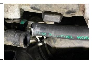
Loosely install one of the provided 90 degree push-lok hose ends to the top fitting of the catch can closest to the firewall. Cut the hose from the previous step to the proper length. Ensure the hose is not kinked or pinched.
