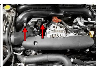
Using pliers, disconnect and remove the hose that runs from the black plastic molded crossover tube to the turbo air inlet pipe. This hose will NOT be reused.
