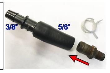
Using light lubrication, install the push-lok hose end into the  $3/8^{\prime\prime}$  hose until all barbs are fully engaged.
