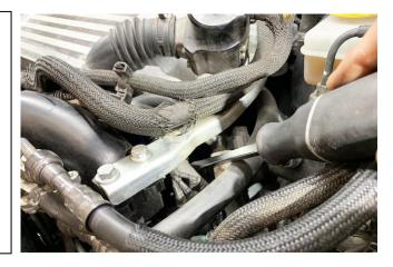
Remove the LH side intercooler bracket. Move the intercooler back and forth to dislodge. Do not lose the turbo outlet gasket on the intercooler inlet. Carefully pull the intercooler upwards and remove from the vehicle.
