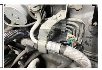
Lineup the included mounting bracket to the 2 threaded holes. NOTE: There is a chance that the lower brake line will need to be slightly adjusted for bracket fitment. Gently pull the hard brake line upwards until the bracket fits without chaffing.
