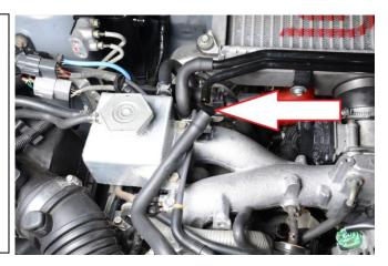
Loosely install both 90 degree 8AN push-lok hose ends to the top and side fittings of the front-most catch can.
