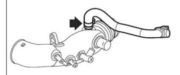
The associated large barbs found on the PCV valve and the 3-way TEE will need to be converted to 3/8" barbs in order to work with the provided 6AN hose end fittings.
