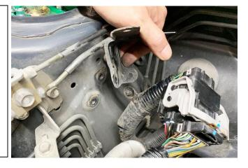
Unlatch the grey lock on the engine harness connector.
