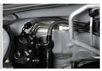
As shown, use the included cable zip-ties to keep the hoses away from moving and/or hot engine parts such as the downpipe and turbocharger.
