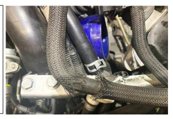
Run the hose towards the TEE fitting and cut to length. Using oil lubrication install the hose to the TEE fitting, as shown.
