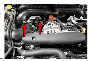
Using pliers, disconnect the hose that runs from the black plastic molded crossover tube underneath the intake manifold to the turbo air inlet pipe.
