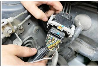
Pully pivot the grey latch. This will disconnect the electrical plug.
