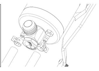
Disconnect the LH side diagnostic connector. Pull the metal shunt out of the diagnostic connector using needle nose pliers.
