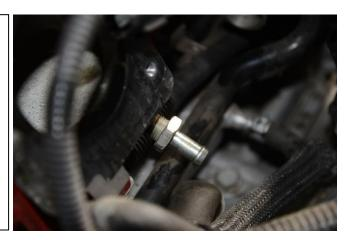
Lubricate the 8AN male O-ring with light oil and tighten into the side port. Lubricate the O-rings on the 2 small hose barb adapters with light oil and tighten into the bottom ports.
