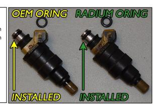
6. If aftermarket injectors are to be used, be sure the upper O-ring seats inside the injector bore. Washer shims (not included) may be required for proper fitment. The fuel injector must have specific spacing, as shown.
