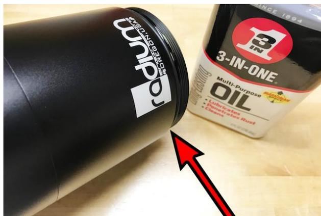
5. Adapter fittings are not provided. Go to [www.radiumauto.com](http://www.radiumauto.com) to find a wide array of 10AN ORB fitting configurations, sizes, and styles. Before installing, make sure to lubricate the O-rings. Aluminum wrenches are recommended to prevent surface marring.
