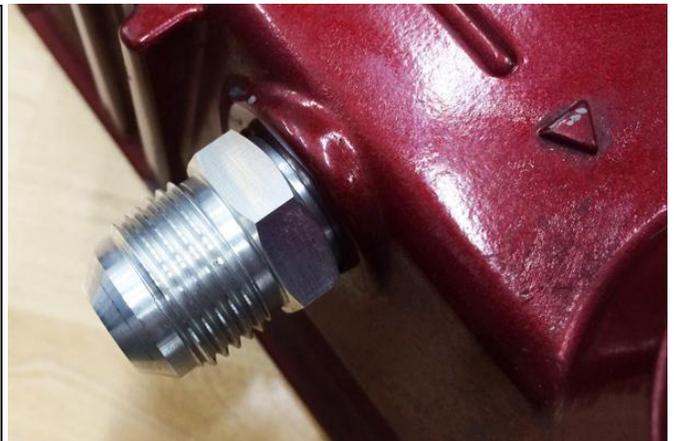
6. When installing a hose end (not included), use a 7/8" wrench on the valve cover fitting to prevent it from spinning.
