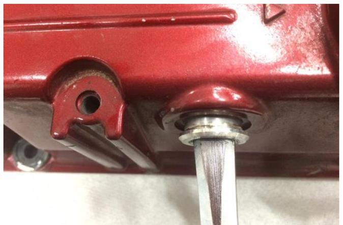
4. A rubber mallet will likely be required to press the included 10AN male fitting into the valve cover hole. Place the fitting in a freezer for 5-10 minutes in an attempt to decrease its size.
