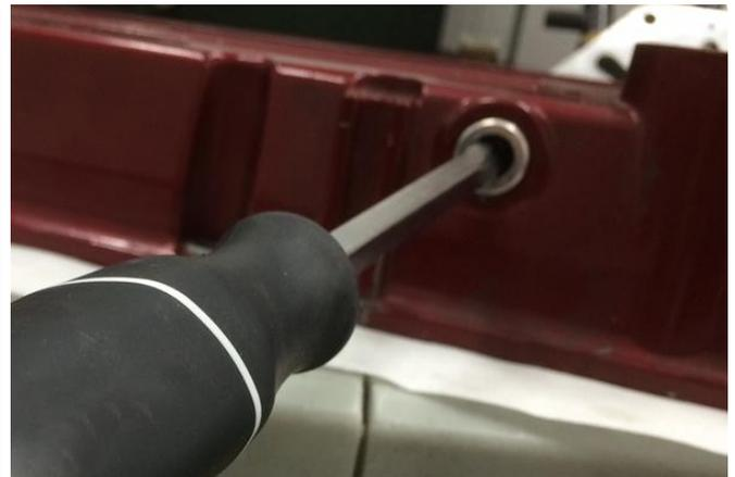
3. Gently move the bushing around and pull, being cautious not to deform the valve cover.
