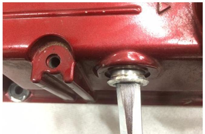
4. A rubber mallet will likely be required to press the included 10AN male fitting into the valve cover hole. Place the fitting in a freezer for 5-10 minutes in an attempt to decrease its size.
