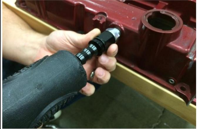
5. The fitting will NOT bottom out onto the hex. There is a machined shoulder allowing it to seat properly into the valve cover hole's recessed area. There will be a small gap (as shown) when properly installed.
