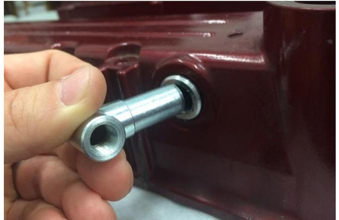
2. NOTE: The aluminum 10AN male fitting cannot be welded to the magnesium Mitsubishi valve cover.
