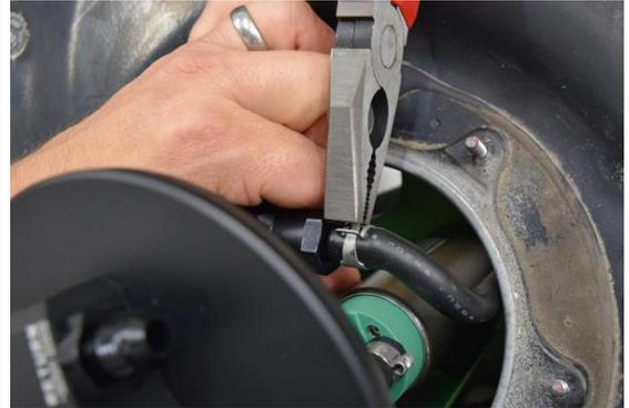
17. Wrap the OEM retaining ring around the hanger top and then carefully drop the hanger down onto the tank. It may be necessary to remove the "Pump Out" fitting to install the retaining ring.
