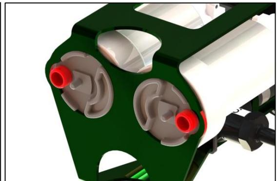
9. Remove the Radium fuel sensor mount attached to the collector box (shown in red). Slide the 2 included zip ties (shown in yellow) in and out of the 4 slotted holes. Using a 3mm Allen wrench, reattach the Radium fuel sensor mount to the collector box using the provided screws.
