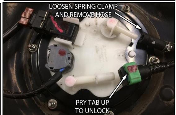
3. To release the OEM fuel pressure sensor, spread the two retaining tabs outwards and simultaneously pull upwards, as shown. Unplugging this connector is not necessary.
