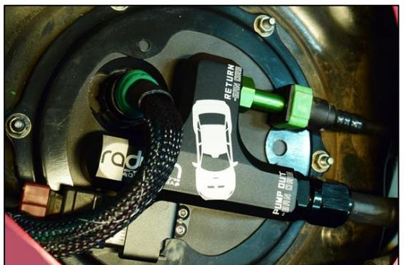
35. Torque the 5/16" SAE Male Fitting into either end of the PTFE hose included in the kit. If installing to a Radium fuel rail with a DMR installed onto the top port, make sure the 6AN male return fitting is pointing towards the left side of the vehicle. Loosely install the opposing hose end to the DMR's 6AN male fitting. NOTE: Hose routing will differ if installing onto a different brand pressure regulator.
