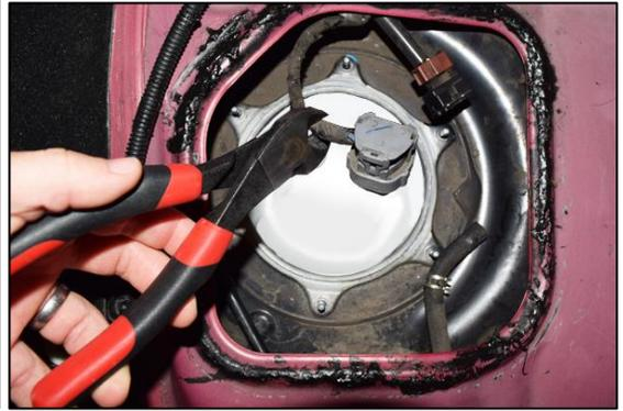
21. Use the large diameter shrink tube and large AWG ring terminals to connect the pump wires ("PWR" for positive and "GND" for negative). Single pump applications use the "Pump 1" terminals. After the ring terminals are positioned on the studs, install the plastic nuts. Then tighten the plastic nuts with a 3/8" driver. Be careful not to over-tighten.
