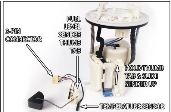
6. **If this kit was shipped from Radium after 9/1/18, this step does not apply and should be skipped. A service-free venturi jet pump was implemented that features a pressure relief valve.**
