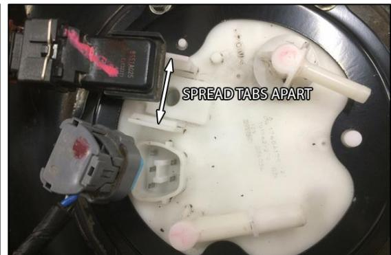
4. Before removing the OEM fuel pump housing, place an empty bucket nearby, there will be residual fuel in the gas tank. Tilt the fuel pump housing towards the right side of the vehicle then pull up. Be careful not to damage the fuel level float arm. Using pliers, release the crossover hose, as shown. Pull the OEM fuel pump housing out and drain into the bucket.
