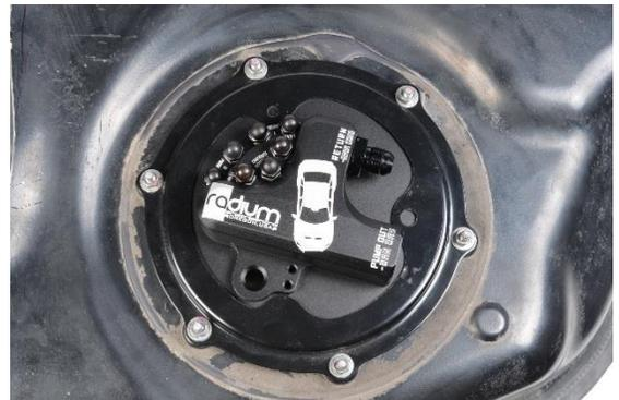
18. The top plate and gasket should be flush with the mounting ring.
