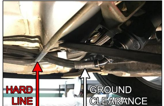
32. Using a 7/8" wrench, torque the 45 degree hose end on the fuel filter inlet first, then torque the straight hose end on the pump hanger. To avoid breaking anything, brace the part. To prevent hose end marring, an aluminum wrench is recommended.
