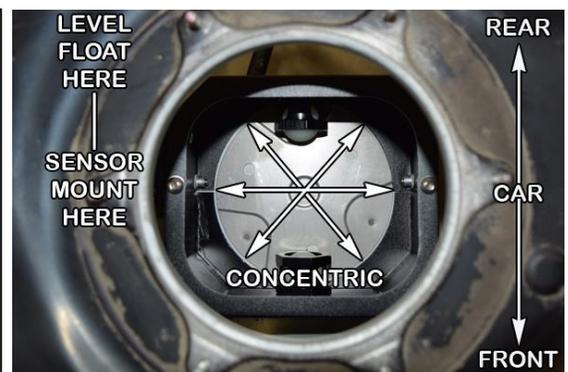
15. Install and fully seat the OEM rubber gasket underneath the fuel pump hanger top plate, as shown.
