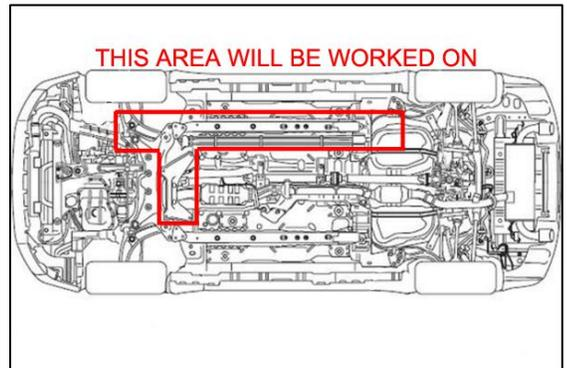
25. The plastic shield (pictured) near the left rear tire and the metal shield near the front left tire that covers the hard lines need to be removed temporarily. Using a 10mm socket wrench, remove the M6 screws and drop the shield down.
