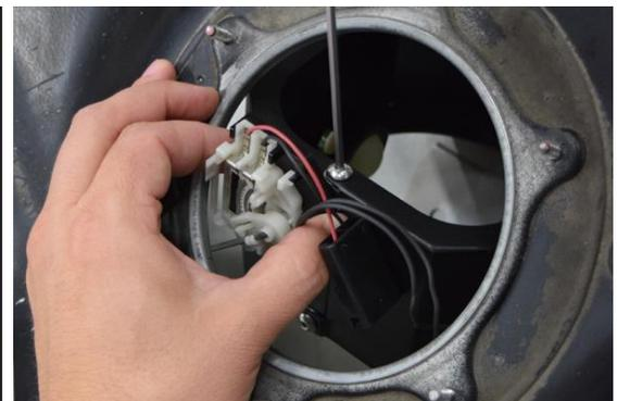
14. Observe the orientation of the collector box in the picture at right.
