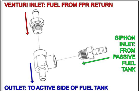
7. To install pumps, the hanger must be partially disassembled. First, remove the 3 internal pump hanger bracket bolts using a 4mm Allen wrench. and replace with the included barb fitting (lubricate O-ring first). Note: The barb fittings (pictured in red) can be used in either port since they share the same outlet.
