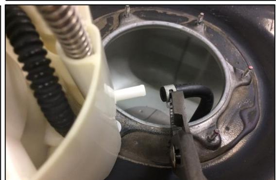
5. To remove the fuel level and fuel temperature sensors from the OEM fuel pump housing, first depress the thumb tab and unplug the 3-pin connector from underneath the top plate. Next, pry and pop the fuel temperature sensor probe out of the securing tabs.
