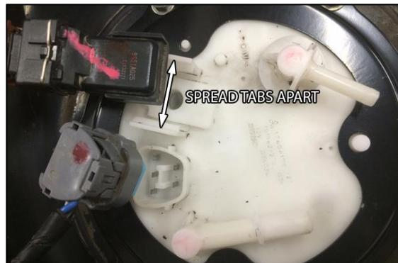
4. Before removing the OEM fuel pump housing, place an empty bucket nearby, there will be residual fuel in the gas tank. Tilt the fuel pump housing towards the right side of the vehicle then pull up. Be careful not to damage the fuel level float arm. Using pliers, release the crossover hose, as shown. Pull the OEM fuel pump housing out and drain into the bucket.
