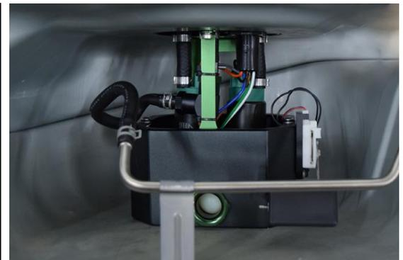
19. Lubricate the O-ring found on the OEM pressure sensor and insert it into the top of the hanger.
