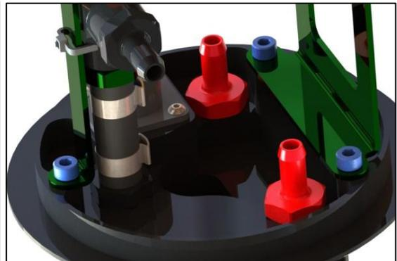
8. Rotate and align the fuel pump(s) concentrically with the cut-outs in the internal pump bracket, as shown in red. Tighten the EFI hose clamps after the alignment is complete. Reinstall the green internal pump bracket. Using the included zip tie, strap the jet pump body to the green bracket. Next, press the filter sock(s) onto each pump inlet and secure with the star washer.
