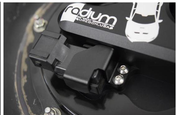
20. **External Wiring:** Cut off the OEM 5-pin fuel pump control module connector, as shown. Remove some of the tape, and wire loom than strip the insulation on all 5 wires about ¼" back.
