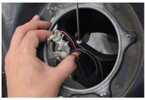
14. Observe the orientation of the collector box in the picture at right.
