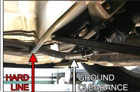
32. Using a 7/8" wrench, torque the 45 degree hose end on the fuel filter inlet first, than torque the straight hose end on the pump hanger. To avoid breaking anything, brace the part. To prevent hose end marring, an aluminum wrench is recommended.
