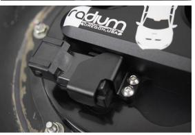
20. External Wiring: Cut off the OEM 5-pin fuel pump control module connector, as shown. Remove some of the tape, and wire loom than strip all 5 wires.
