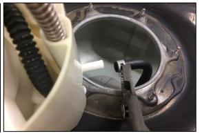
5. To remove the fuel level and fuel temperature sensors from the OEM fuel pump housing, first depress the thumb tab and unplug the 3-pin connector from underneath the top plate.
