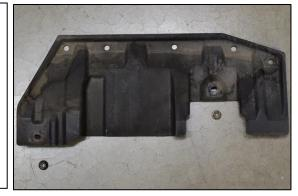
26. The center metal under tray brace (pictured) under the exhaust downpipe elbow and driveshaft needs to be removed temporarily. Remove the 4 bolts and drop the brace down.
