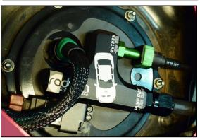
35. Torque the 5/16" SAE Male Fitting into either end of the PTFE hose included in the kit. If installing to a Radium fuel rail with a DMR installed onto the top port, make sure the 6AN male return fitting is pointing towards the left side of the vehicle. Loosely install the opposing hose end to the DMR's 6AN female fitting. NOTE: Hose routing will differ if installing onto a different brand pressure regulator.
