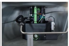
19. Lubricate the O-ring found on the OEM pressure sensor and insert it into the top of the hanger.
