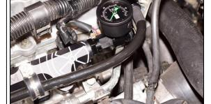
36. NOTE: This kit eliminates the OEM hanger's "post" fuel pump filter so a low micron aftermarket filter should be installed downstream to protect the injectors from debris.
