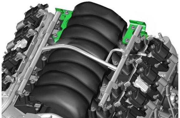
9. The 20-0232 fuel rails do not include plumbing. NOTE: Early LS1 engines (97-99) will require an aftermarket FPR to replace the regulator on the OEM rail. The Radium Engineering direct mount regulator (DMR) is shown as an example.
