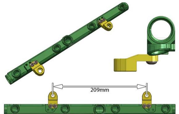
4. For intake manifolds which have 224mm spacing between the 2 fuel rail mounting bosses, install the mounting feet using the outer threaded holes and flip them so they are short, as shown.
