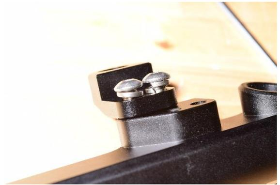
6. Prepare to install the necessary adapter fittings into each fuel rail port. **To avoid damage, lubricate all O-rings with oil prior to installing.**
