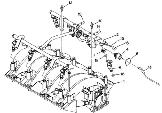
3. The included mounting feet allow installation of OEM injectors on various LS style intake manifolds. For instance, flipping the mounts over affects rail height. Securing them to the rail in specified holes affects fuel rail mount spacing.
