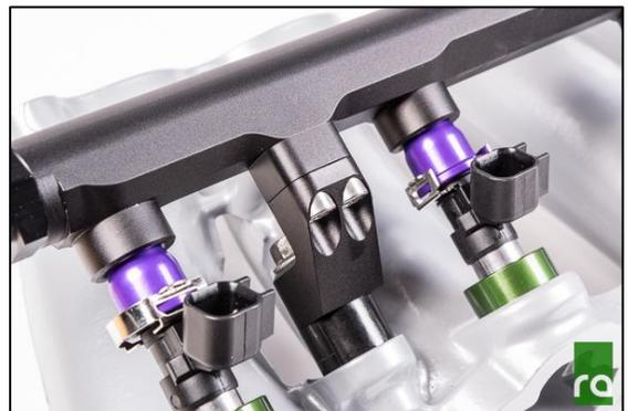
8. **Using the OEM fuel rail spacers**, position the fuel rail assembly on the intake manifold. Install the OEM M8 bolts and torque to 15ftlbs (21Nm) using a 12mm socket wrench.
