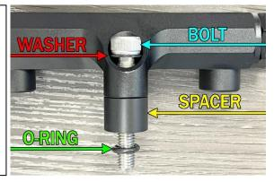
6. As shown, squeeze everything together. This will prevent any hardware from falling and getting lost in the engine bay. Place the fuel rail on the lower intake manifold.
