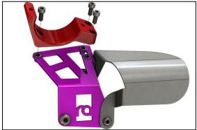
7. Temporarily install the Radium fuel filter (not included) and upper clamp to the lower mount using the 2 socket head screws and a 4mm Allen wrench. Do not torque these bolts yet.
