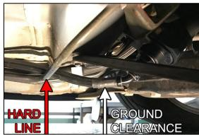
10. When reinstalling the center under tray brace, first check for clearance near the hose end to the fuel filter inlet. Grind if necessary.
