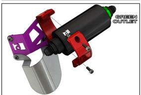
8. From underneath the vehicle, pull and slide the fuel filter downwards out of the clamp. Torque the hose end (not included) to the green fuel filter outlet. Slide the fuel filter all the way back into place. Lineup the clamp to the filter, as shown. For hose end clocking purposes, allow the filter to rotate inside the clamp.
