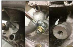
7. **Lubricate all adapter fitting O-rings** and secure to the three 8AN ORB ports (Radium fuel pulse damper shown).
