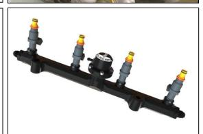
8. Using the OEM insulating spacers (16638-PNA-000), position the assembly onto the manifold. Check for clearances issues and grind, if necessary. Torque the included M8 bolts and washers to 10 ft-lbs (13.6Nm) using a 6mm Allen wrench.
