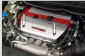
3. Disconnect the 4 fuel injector connectors.
