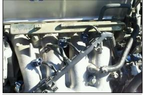
4. A few of the OEM fuel rails came standard with a fuel pulse damper. If the engine did not come with this fuel rail, skip to the next step.
