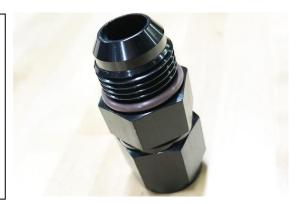
26. Apply Teflon paste to the fuel pressure gauge threads and screw it into the inline 1/8" NPT adapter fitting. Tighten finger tight, then add another 1.5 to 3 turns with a wrench.
