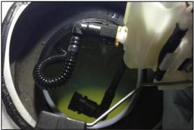
5. The only part that will be reused from the housing is the fuel level sender and the large gasket.
