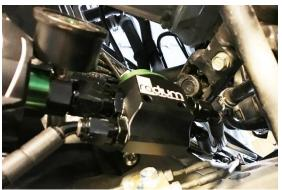
29. Secure the fuel filter heat exchanger section of the assembly to the mounting bracket using the four included M6 socket head bolts. Tighten using a 5mm Allen hex wrench.
