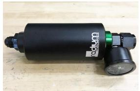
27. Slide the fuel filter into the heat exchanger. Using a 4mm Allen hex wrench, secure the heat exchanger to the filter by tightening the M5 flat head screws.
