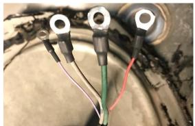
22. Optional high-current wiring: For high flow, high pressure fuel pumps, consider using Radium DIY wiring kit 17-0031 (shown) for each pump. This includes a dedicated fuse, relay, 10AWG wire, etc. It is recommended to use the OEM fuel pump wiring to trigger this fused relay power source for each pump.
